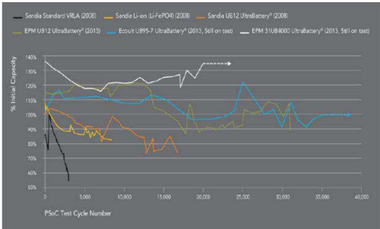
Figure 8: Longevity test of VRLA battery, Li-Ion battery, and UltraBattery for regulation service application PSoC 68
