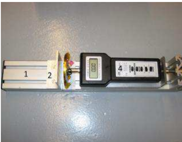
Figure 28: Jig for the quantitative control of an electrode cell compression: 1- base, 2- blocker, 3- pusher, and 4- digital controller of work loading.
