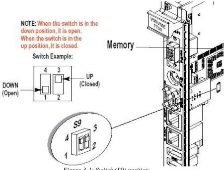
Figure 3-1: Switch (S9) position
