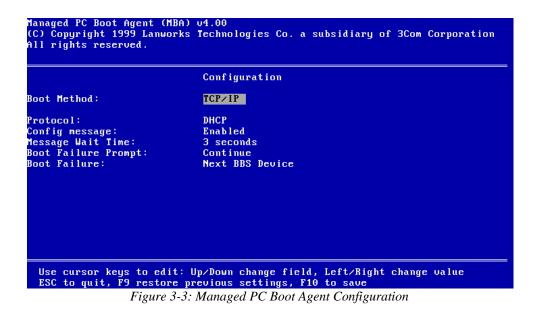
The Boot Method should be set to PXE. Once you have made the change, press F10 to save the configuration and exit.
