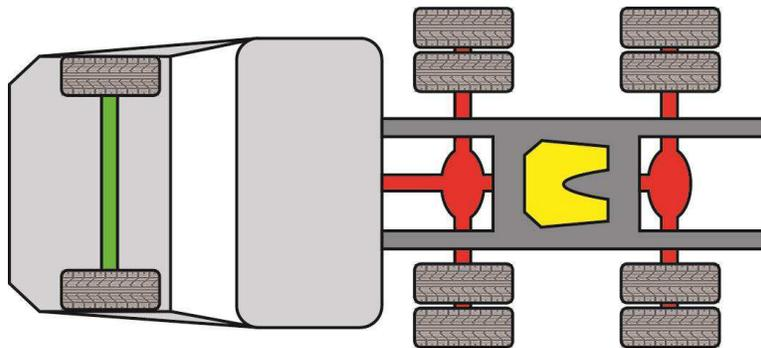
Figure 1: 6x4 arrangement (adapted from [1])
