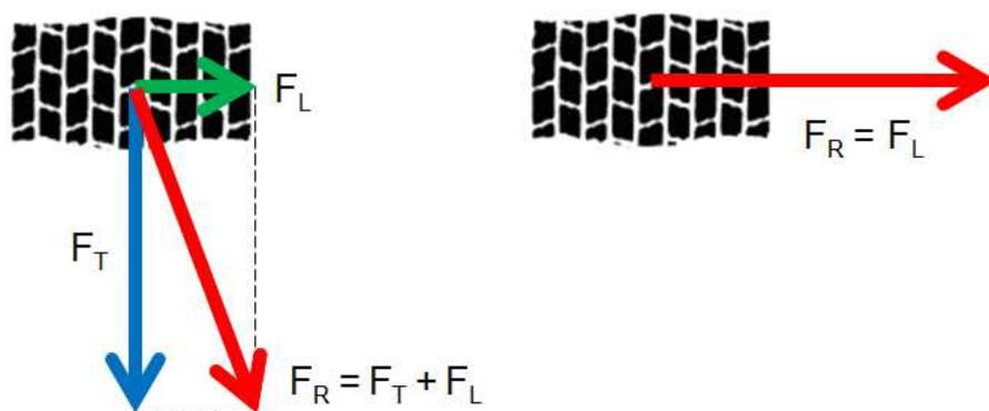
**Figure 16: Available lateral stability between powered and non-powered tire**
