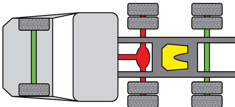
Figure 2: 6x2 tag tandem 6x2 architecture [1]
