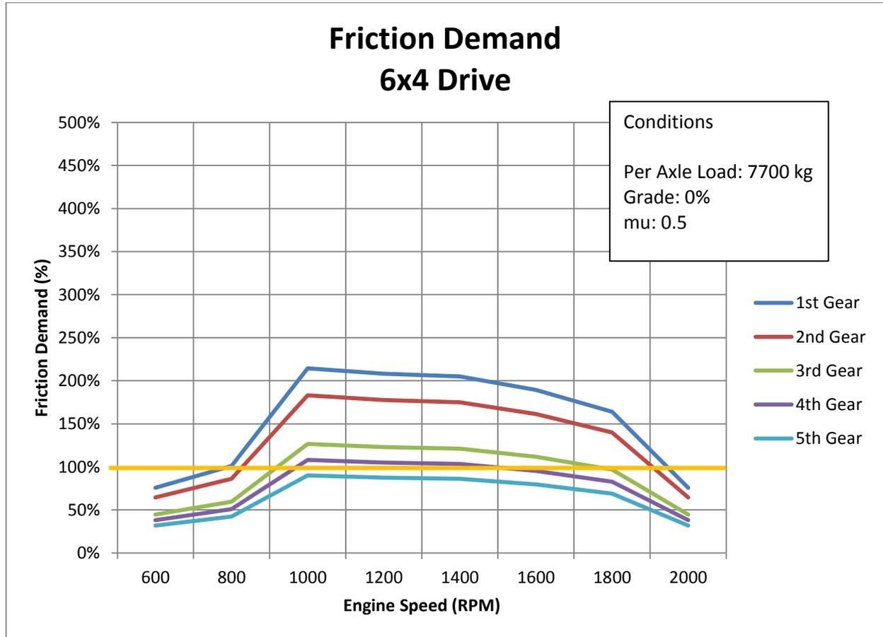
Figure 8: 6x4 friction demand (7,700 kg axle load, 0% grade, mu of 0.5)
