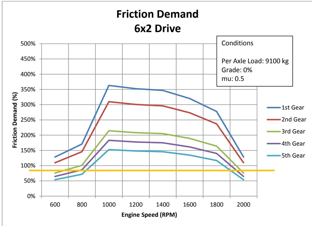
**Figure 14: 6x2 friction demand (9,100 kg axle load, 0% grade, mu of 0.5)**
