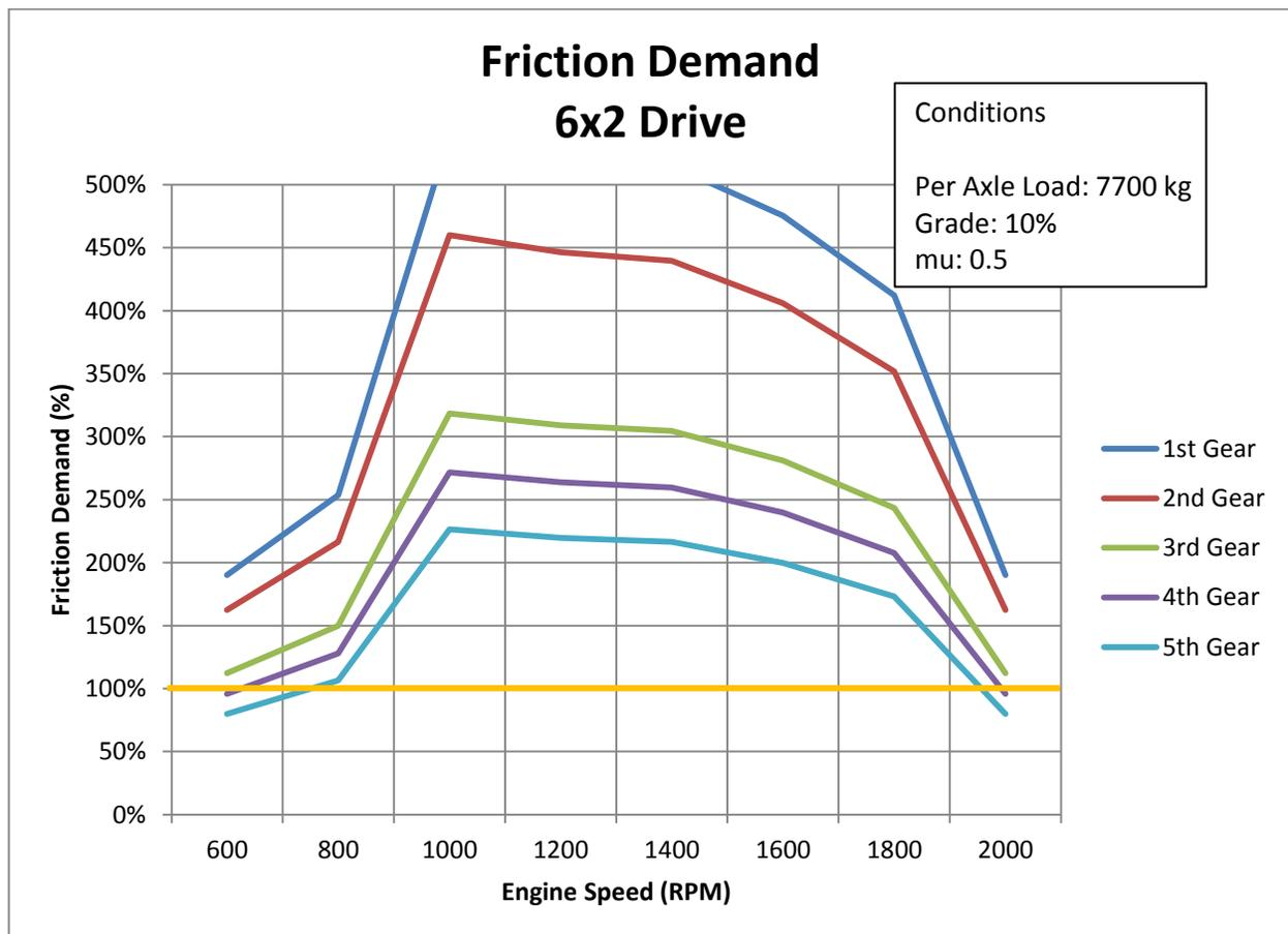
Figure 9: 6x2 friction demand (7,700 kg axle load, 10% grade,  $\mu$  of 0.5)
