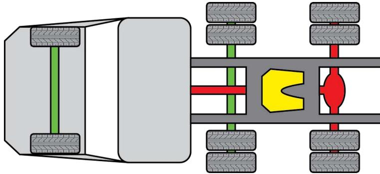
**Figure 3: 6x2 pusher tag 6x2 architecture [1]**
