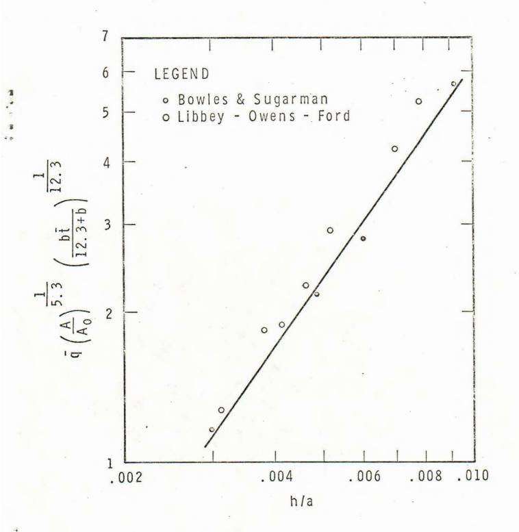
CORRELATION OF STRENGTH OF UNIFORMLY LOADED SQUARE GLASS PLATES FROM TWO INDEPENDENT SOURCES (SODA-LIME PLATE GLASS)
