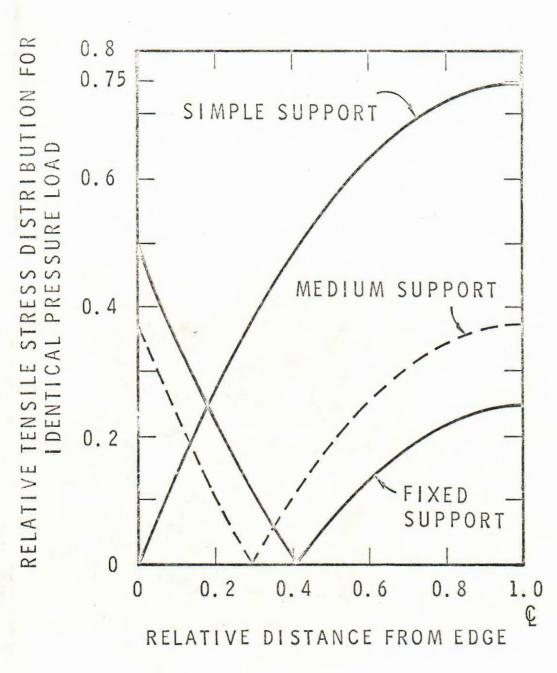
TENSILE STRESS DISTRIBUTION IN RECTANGULAR PLATES SUPPORTED ON TWO OPPOSITE SIDES. (CORRESPONDS TO LONG NARROW PLATES)
