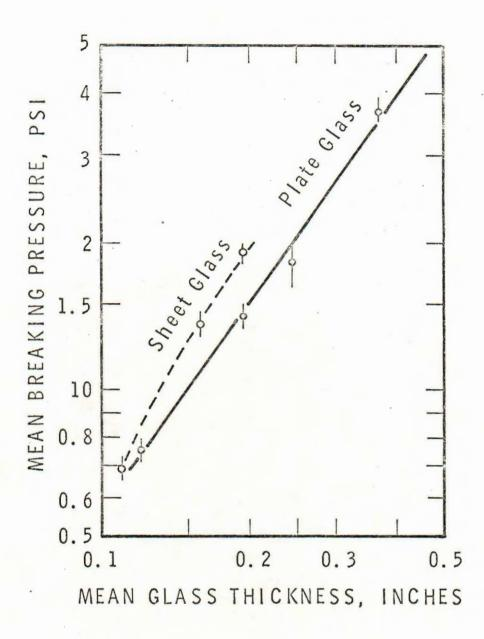
MEAN BREAKING PRESSURE AS DEPENDENT ON PLATE THICKNESS. SIMPLY-SUPPORTED SQUARE PLATES, (BOWLES & SUGARMAN)
