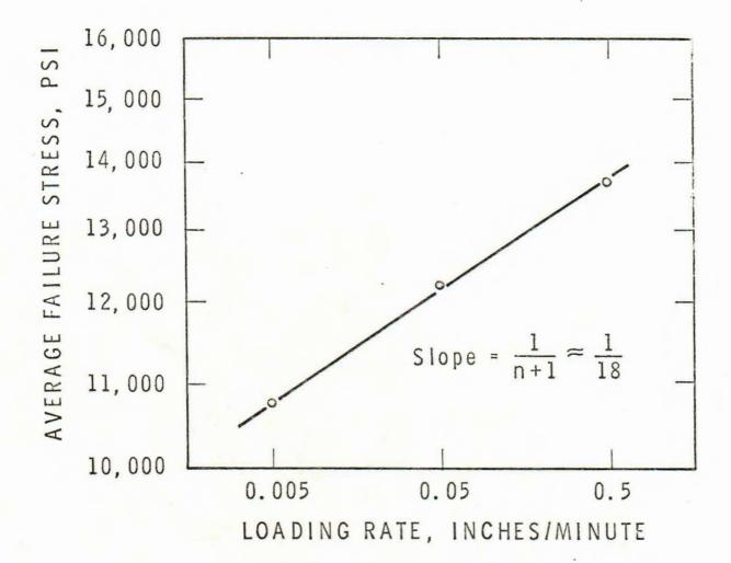
EFFECT OF CONSTANT LOADING RATE ON AVERAGE FAILURE STRESS AT 25°C (After Charles (4))
