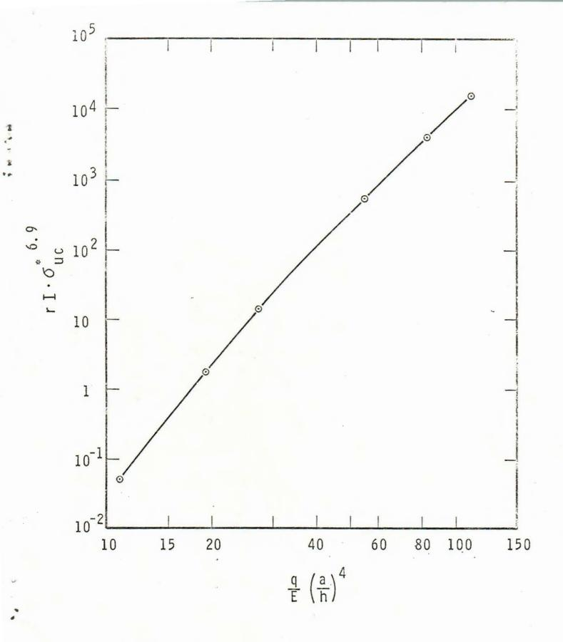
PROBABILITY PARAMETERS DERIVED FROM STRESS DISTRIBUTION DATA OF KAISER (18). SIMPLY SUPPORTED SQUARE GLASS PLATE.
