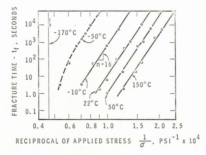
EXPERIMENTAL RESULTS FROM STATIC FATIGUE TESTING OF SODA LIME GLASS RODS (CORNING 0080) IN SATURATED WATER VAPOR. AFTER CHARLES (3)
