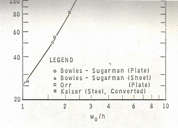
LOAD DEFLECTION RELATIONSHIP FOR UNIFORMLY LOADED, SQUARE GLASS PLATES WITH SIMPLE SUPPORT
