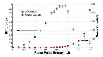
FIG. 3. OKS efficiency (left ordinate: green squares) and noise counts per second (right ordinate: red circles) with respect to the energy of the pump pulse. Error bars on the noise counts are  $\sim \pm 1$  and smaller than the dots shown.
