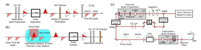
FIG. 1. (a) Schematic diagram for time-bin qubit preparation starting with a polarization state and (b) conversion of time-bin qubits to the polarization degree of freedom by using the OKS. (c) Corresponding experimental setup.
