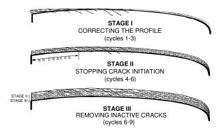
$\label{thm:conditional} \textbf{Figure 2: Staged Crack Removal with the Preventive-Gradual Strategy}$
