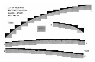
Figure 6: Distribution of surface cracks in a sharp-curve high-rail under preventive grinding.
