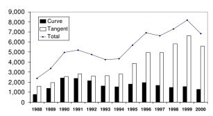
Figure 1: Total Main Track Detail Fractures on BNSF By Year.
