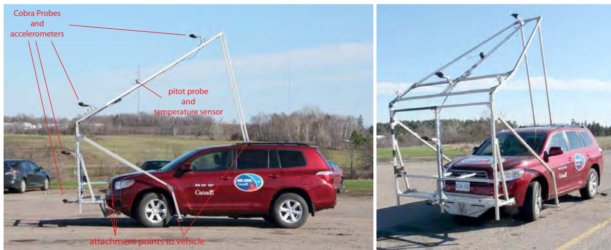
Figure 1.3: SUV with support rig for on-road turbulence measurements (left - side view, right - front view)
