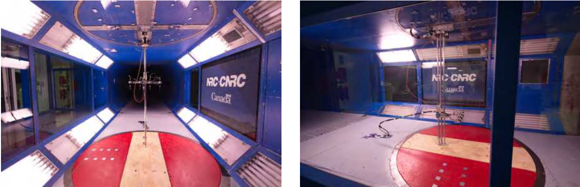
Figure 5.2: Left: Downstream view of the vertical traverse for measurements at the centre of the test section with the 4 Cobra probes mounted on a horizontal bar and spaced by 15 cm. Right: Side view of the vertical traverse during wind on measurements
