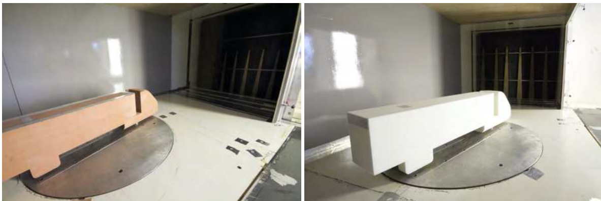
Figure 1.5: HDV models and FTS concepts in NRC NRC 1.0 m \times 0.8 m Pilot Wind Tunnel (left - pressure model with short spires, right - lightweight model with tall spires)
