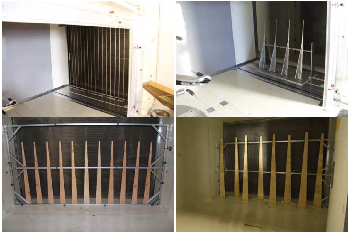
Figure 1.4: Passive techniques examined to for turbulence generation in the NRC 1.0 m \times 0.8 m Pilot Wind Tunnel: vertical bars + screen (top left), moving spires (top right), short and narrow settling-chamber spires (bottom left), tall and staggered settling-chamber spires (bottom right)
