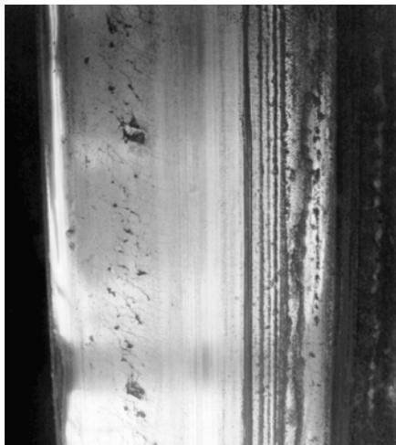
**Figure 7: Cracked wheels show clearly defined failures repeated around at least most of the circumference.**
