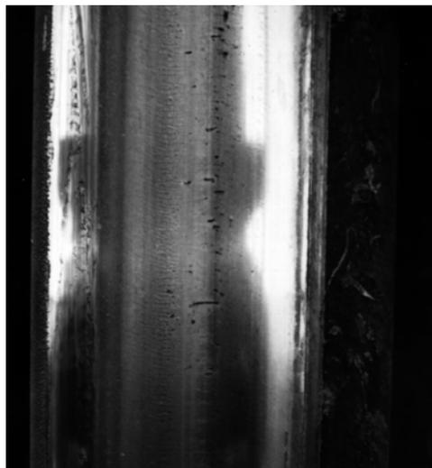
**Figure 8: Thermal cracks showing face separation and axial orientation.**
