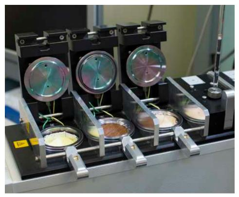
Micro-chamber used for screening VOC emissions from solid building materials
