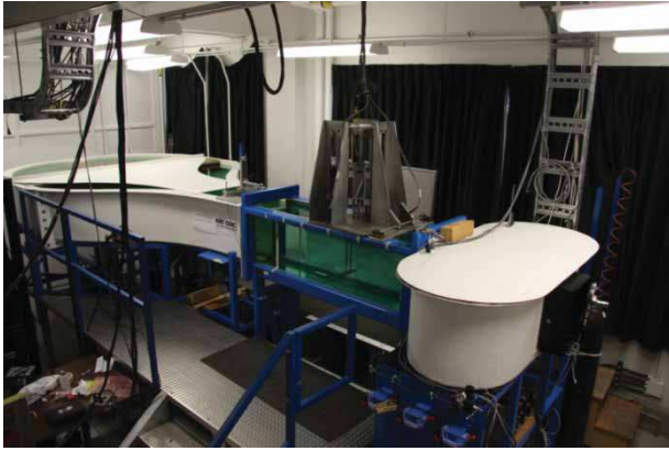
Figure 5. The water tunnel at NRC-Aerospace with the two-axis motion system installed.
