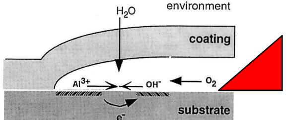
Initiation through a slight corrosion of the aluminum substrate through the penetration of a small amount of water and salt at a defect of the organic coating.
