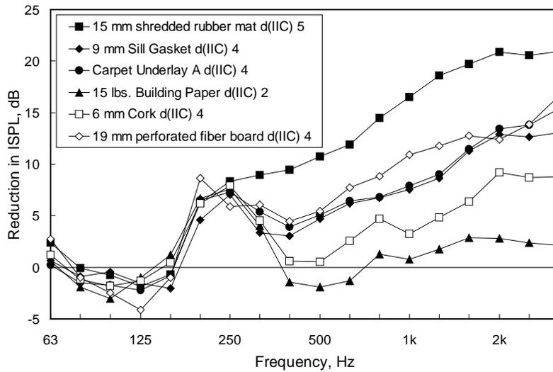
Figure 24: OSB/Steel joist base floor: Various resilient materials tested under a 1.2 x 1.2 m piece of 15 mm thick OSB.  $d(IIC)$  is the change in IIC relative to the floor with no topping.  $d(IIC)$  is the change in IIC rating relative to the floor without the topping.
