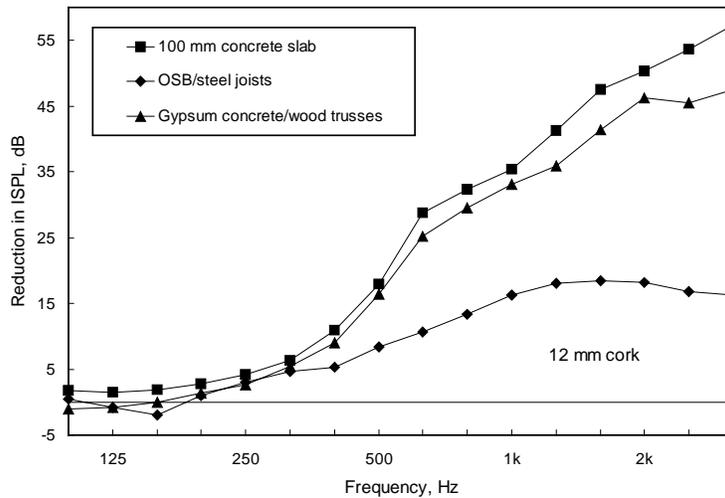
Figure 12: Reduction in impact sound pressure level obtained with 12-mm cork on three floors.
