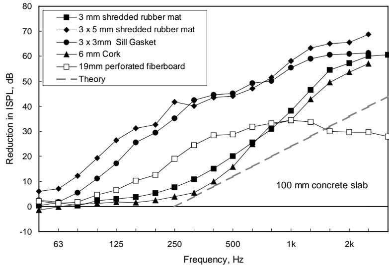
Figure 15: Reduction in impact sound pressure level for different resilient materials placed on top of the 100 mm thick concrete slab.
