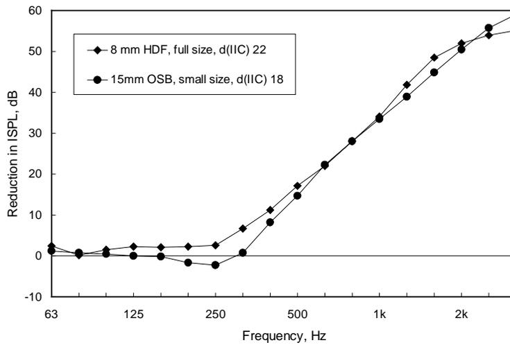
Figure 29: 5 mm shredded rubber mat tested under 8 mm high-density fiberboard (full-size) and under 15 mm OSB (small size).  $d(IIC)$  is the change in IIC rating relative to the floor without the topping.
