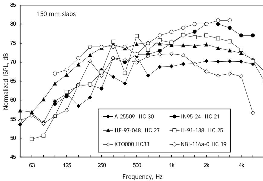
Figure 3: Normalized impact sound pressure levels for 150-mm concrete slabs from different laboratories.
