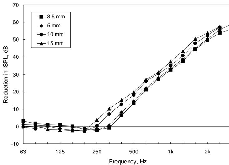
Figure 21: Reduction in impact sound pressure level for four thicknesses of shredded rubber mat under 15 mm OSB placed on the 100 mm concrete slab.
