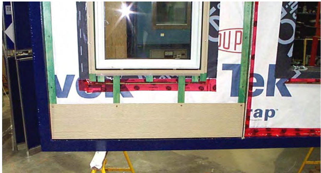
Figure A4-17: Detailing at the sill of the wall/window interface. Same for both halves of the Specimen
