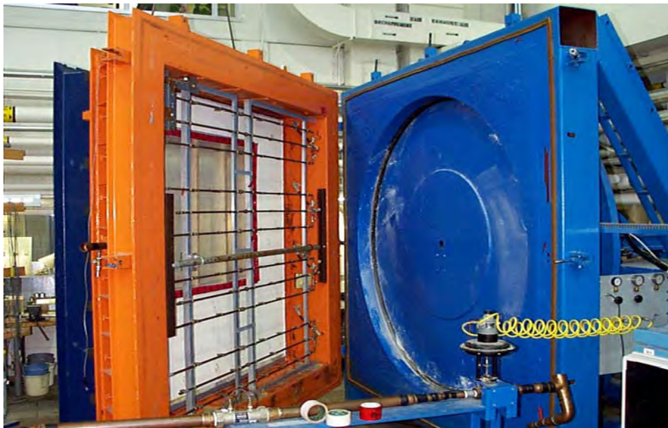
Figure 3-5: Inside view of apparatus showing orange test frame door onto which is affixed test specimen. This same frame contains water spray rack; individual water lines can be seen in photo. When test frame is closed and sealed to test rig, exterior cladding faces inside of apparatus (on right, coloured blue).
