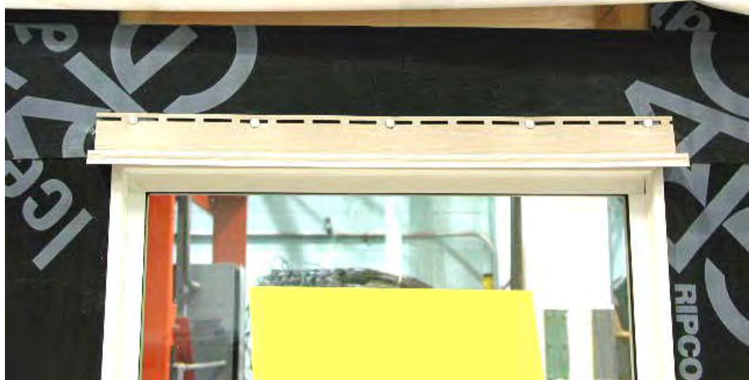
Figure A5-13: Specimen W2 B-side – Placement of the rigid head flashing (drip cap), extending 25 mm (1 in.) on each side
