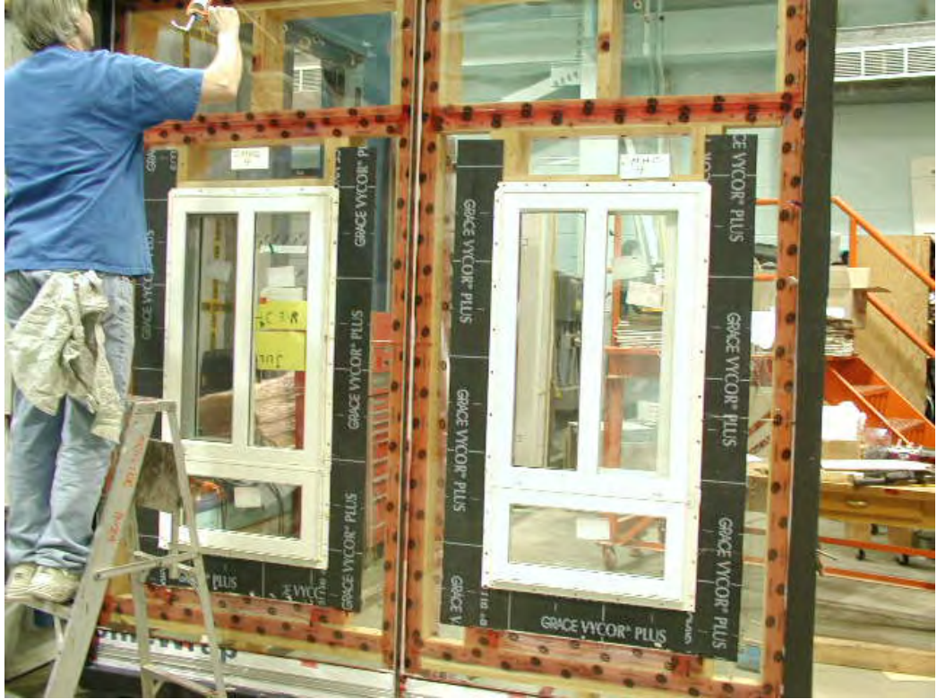
Figure A7-22: Modified Specimen W4 – Installation of the self-adhered membrane on both sides of Specimen
