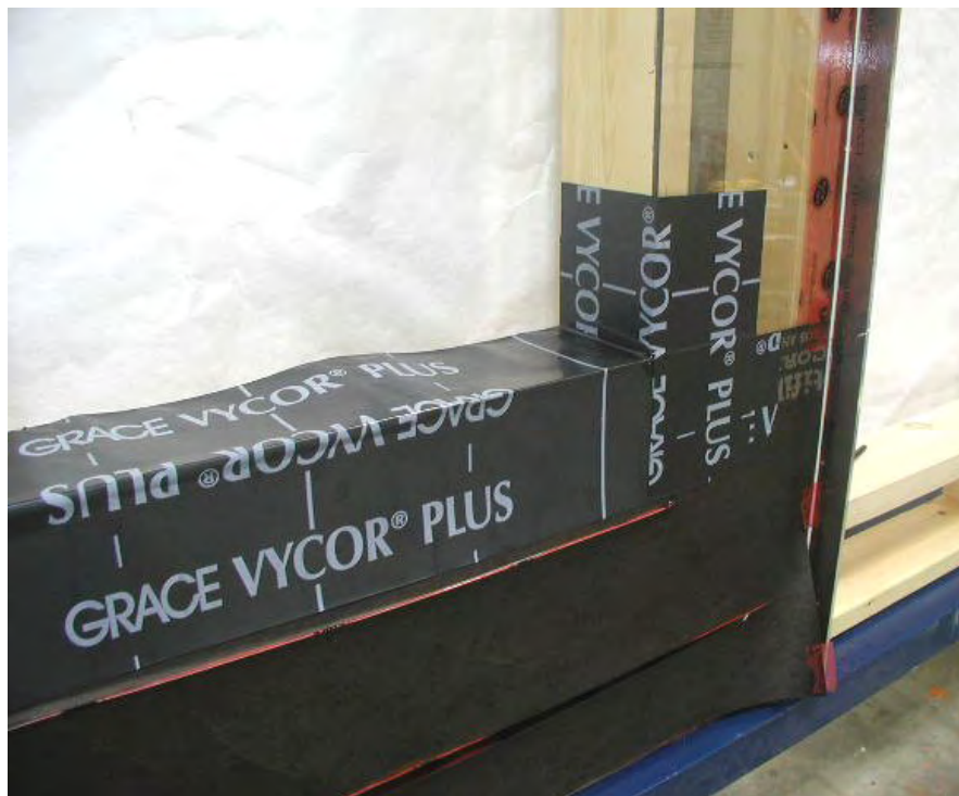
Figure A6-13: Specimen W3 B-side – Strip of waterproof membrane installed at jamb (150-mm high), lapping over the sill membrane
