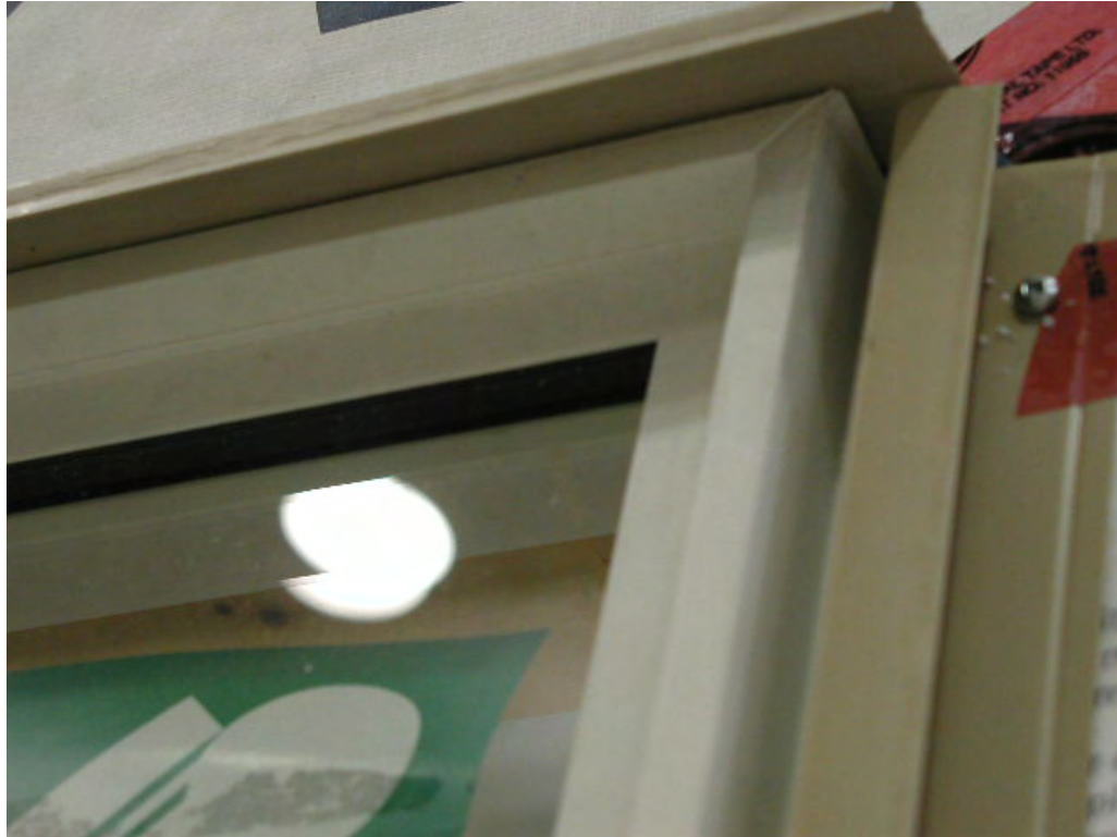
Figure A5-22: Specimen W2 V-side – View of the frame corner, drip flashing and J-trim, prior to installation of backer rod and sealant
