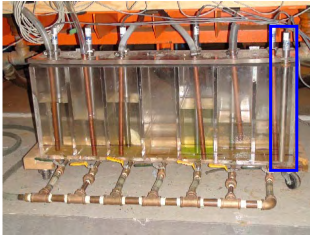
Figure 3-7: Bank of seven (7) calibrated water collection vessels; level sensor is shown on right of photo
