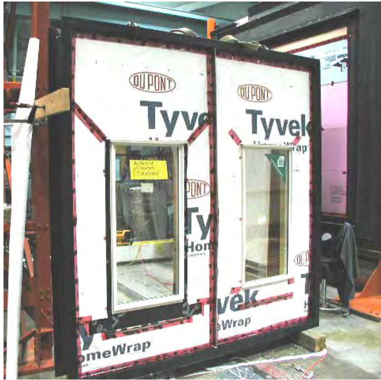
Figure A5-14: Specimen W2 B-side (left of photo) – Water resistive membrane installation completed
