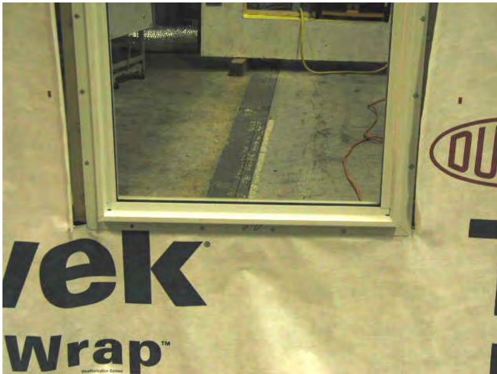
Figure A5-21: Specimen W2 V-side – Window flange is over the WRB at sill, and under the WRB at the jambs and head
