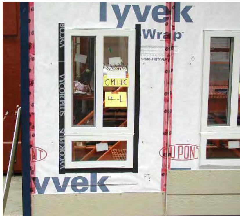
Figure A7-13: Specimen W4 B-side only: Installation of a strip (50-mm) of waterproof membrane sealing the WRB to the window flange
