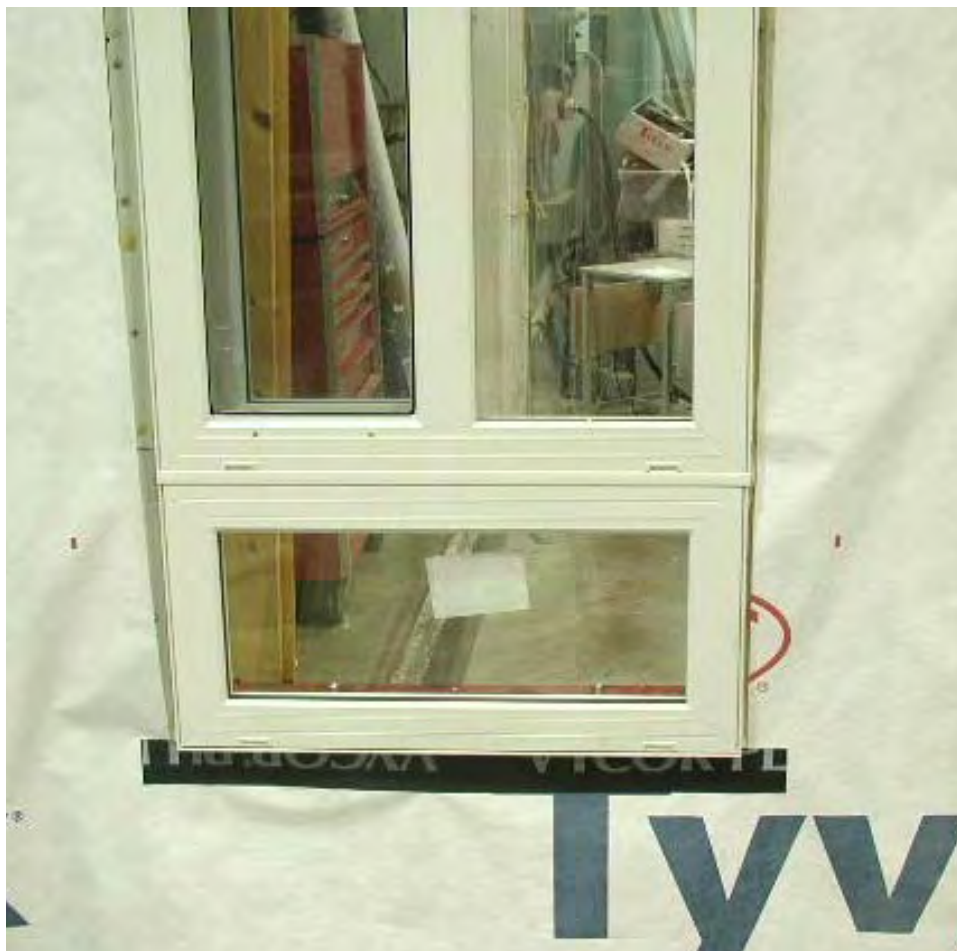
Figure A7-26: Modified Specimen W4 B-side – Self-adhered flashing membrane at sill
