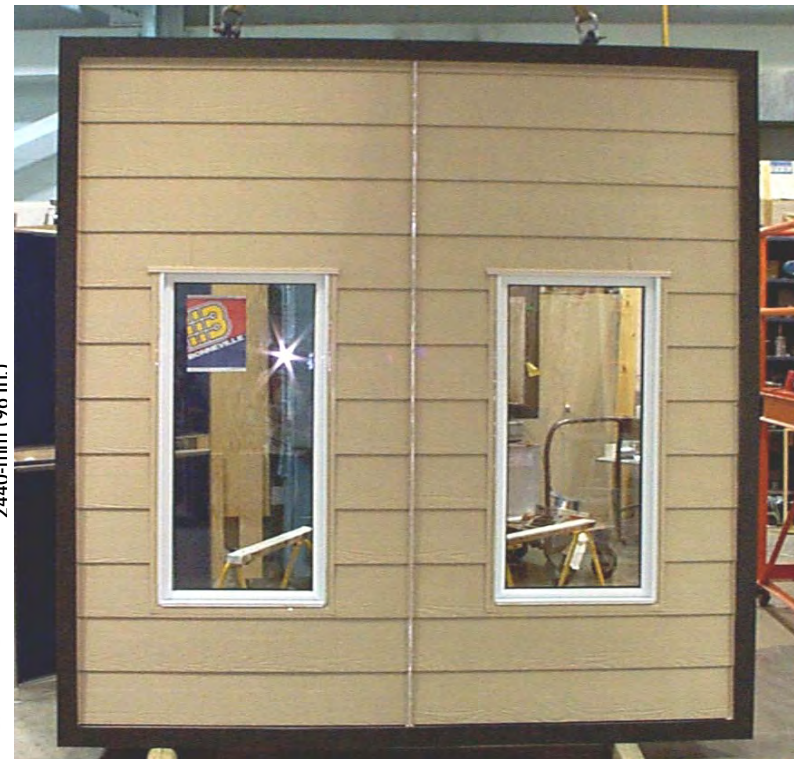
Figure A3-1: Typical layout of the wall Specimen for comparative investigation of the water management response of two side-by-side wall/window interface details (left). Elevation view of the exterior cladding of the Specimen completed (right).
