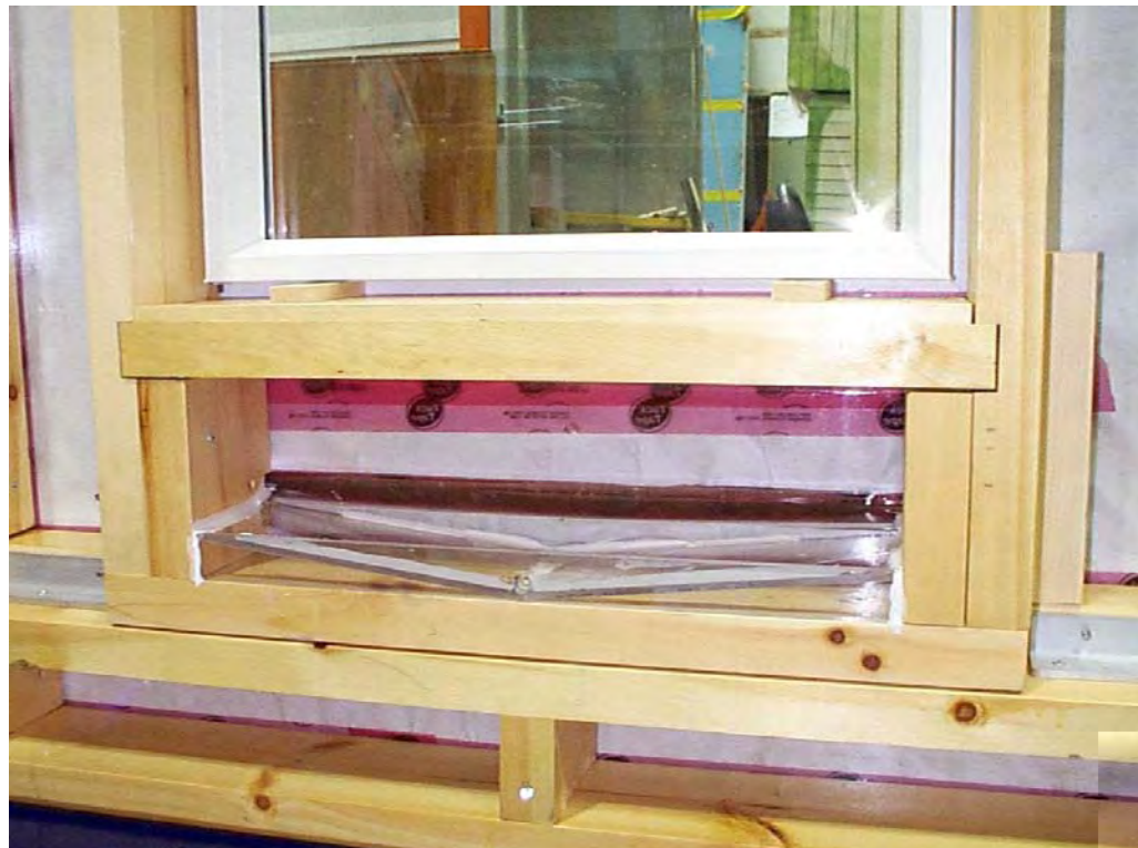
Figure A5-23: Specimen W2 V-side – View of the trough used to collect water
