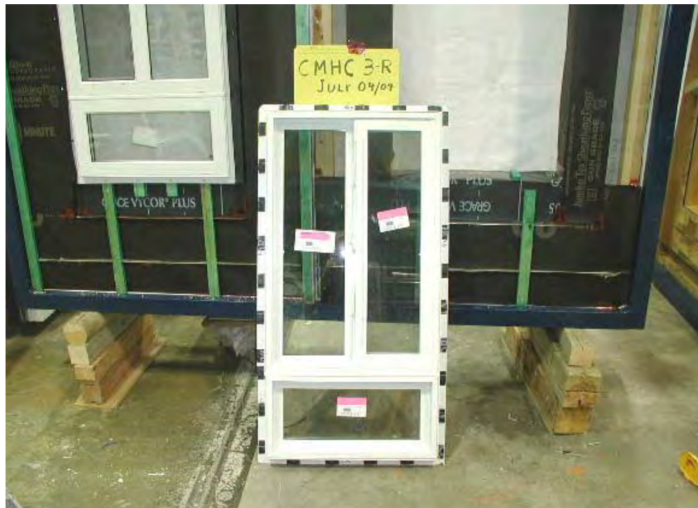
Figure A6-20: Window flange with spacers, designed to create a drainage space at the rough sill (Specimen W3 V side only)
