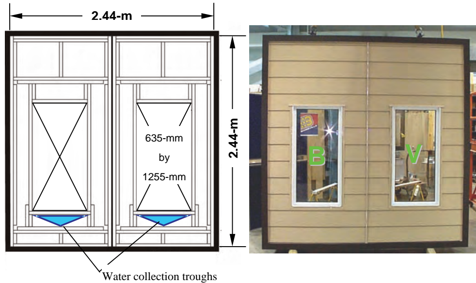
Figure 8-1: (Left) Typical layout of wall specimen framing for investigation of water management response of two side-by-side wall-window interface details (B and V-sides). Water collection troughs are located beneath the windowsill. (Right) Elevation view of exterior cladding of specimen
