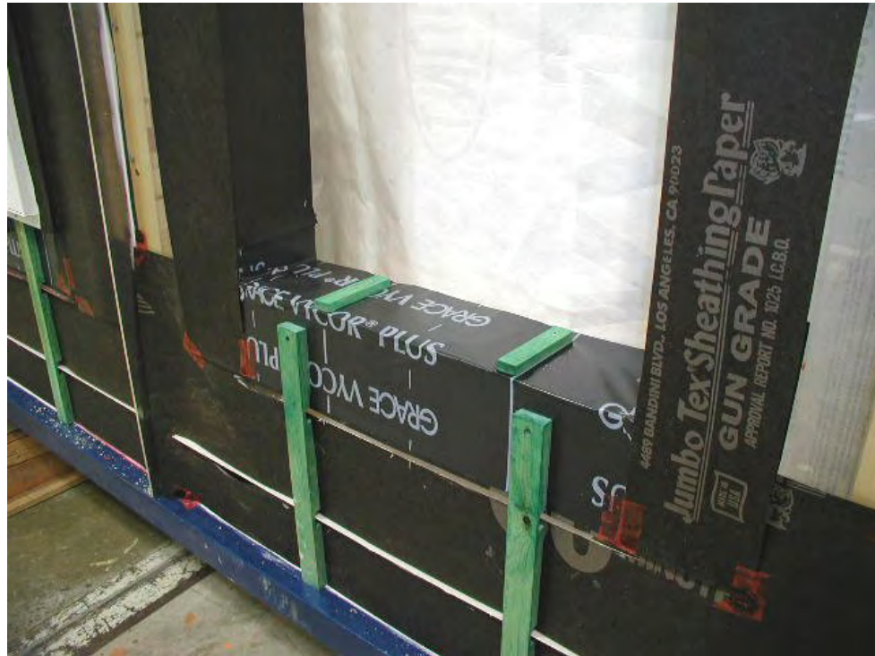
Figure A6-19: Specimen W3 B side: installation of furring strips (19 mm) and shims (12 mm)
