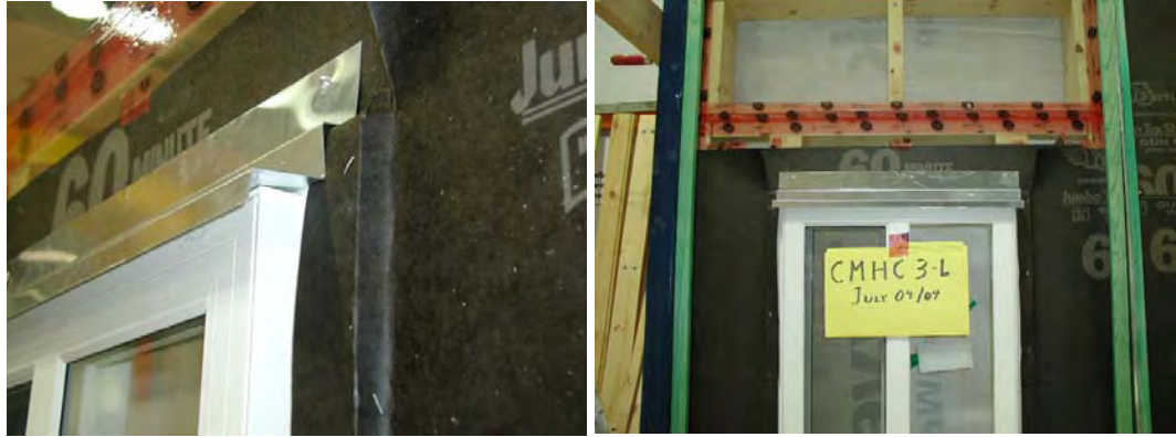
Figure A6-17: Stepped drip cap flashing accommodates window recessed from the back up wall (Specimen W3 B side)
