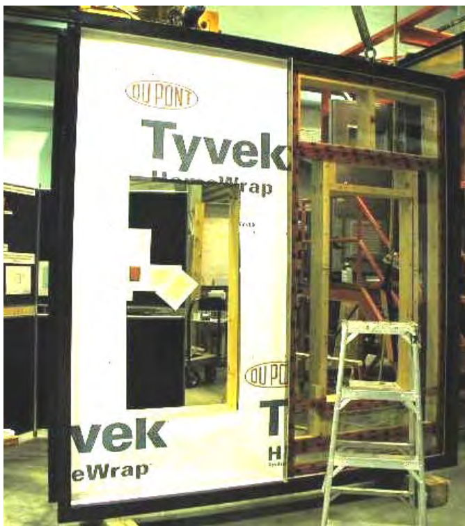
Figure A4-9: Membrane in place cut at the perimeter of the rough opening
