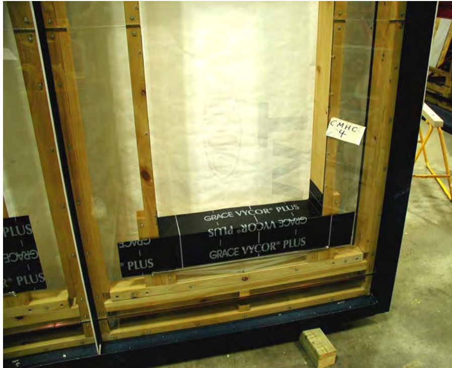
Figure A7-8: Installation of waterproof membrane at the rough sill
