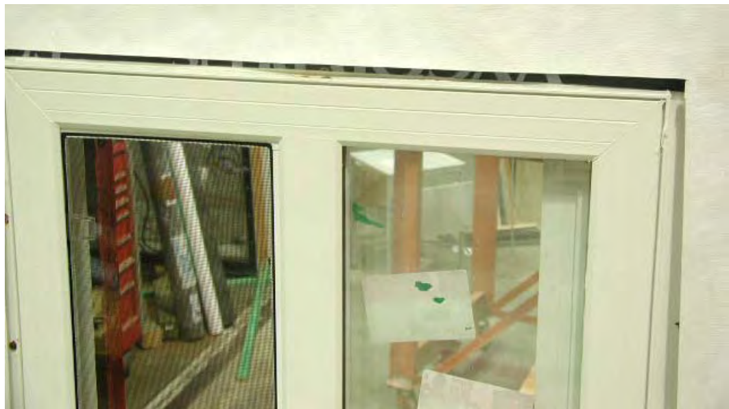
Figure A7-25: Modified Specimen W4 V-side – WRB membrane cut 6 mm short of window frame
