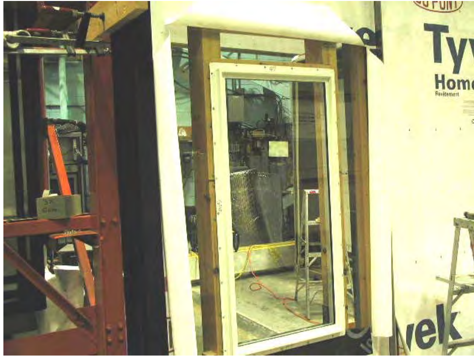
Figure A5-10: Specimen W2 B-side – Fastening of the flanged window to the structure, over the clear acrylic sheet acting as sheathing board
