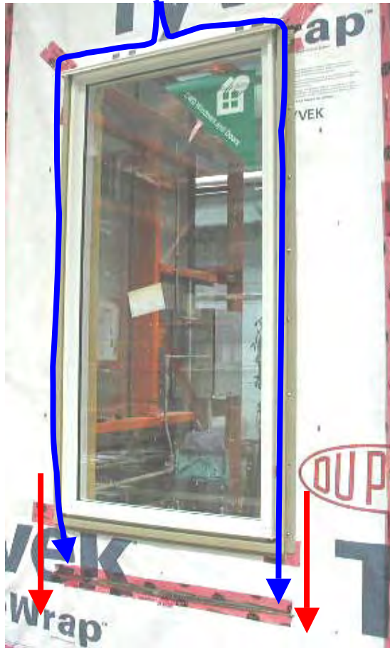
Figure 5-14: Potential path of water to reservoir collection tray during test Trial 3
