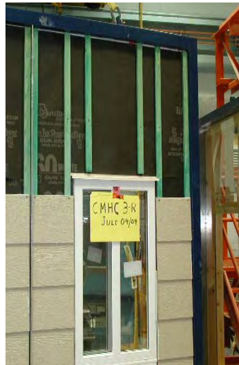
Figure A6-22: Installation of siding on Left and Right sides of Specimen. Siding back-primed and painted (one coat).
