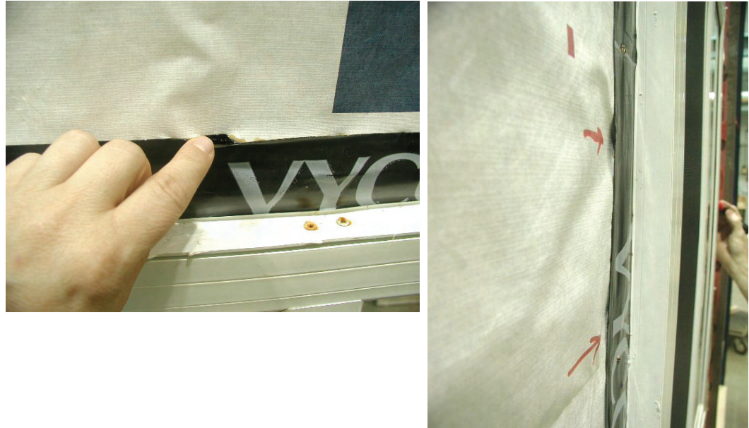
Figure 8-7: Location of delamination, and in some cases, loss of cohesion between plies of the self-adhered flashing membrane
