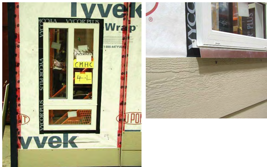
Figure A7-15: Specimen W4 B-side – Self-adhered membrane installed at the perimeter of window frame and WRB junction
