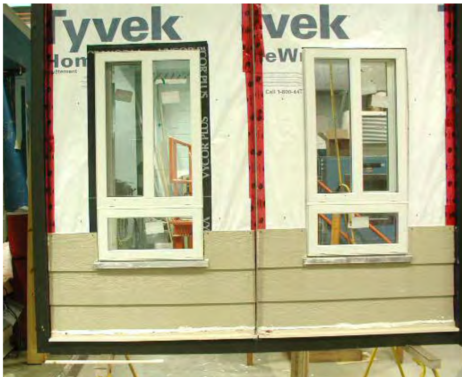
Figure A7-29: Modified Specimen W4. Siding installation (b-side on the left and V-side on the right)
