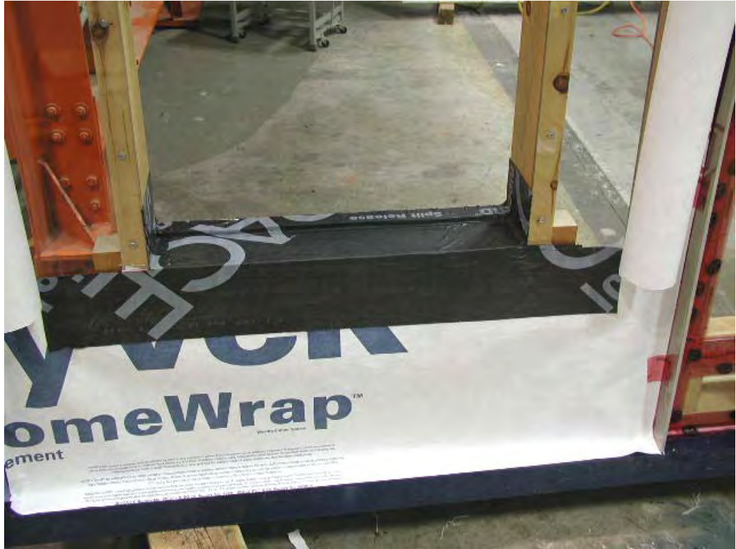
Figure A5-8: Specimen W2 B-side – Detail at sill and lower part of jamb
