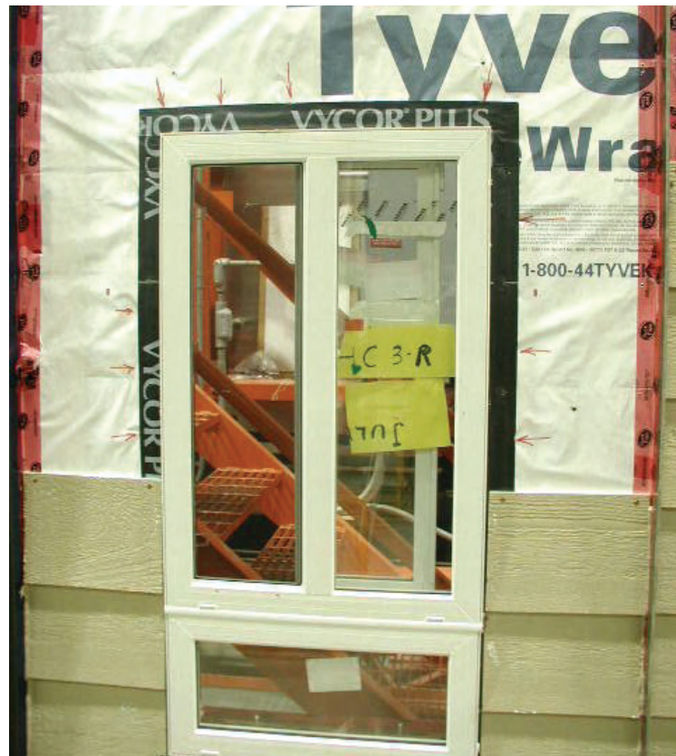
Figure 8-8: Locations (red arrows) along the interface between the window and sheathing board where the flashing membrane delaminated from the sheathing membrane and formed funnels in which water accumulated
