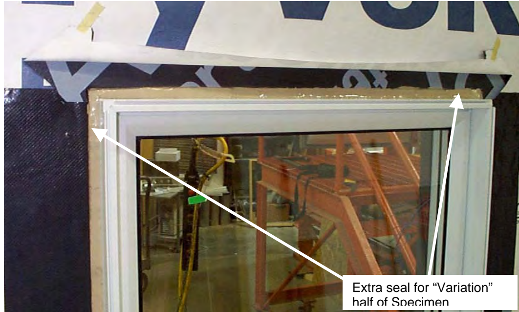
Figure A4-25: Additional sealant and backer rod was placed at the jambs and head of the junction between the window frame and the waterproof membranes, in the plane of the sheathing board. This intends to provide a secondary seal against water entry in case the external bead of sealant fails during service life.
