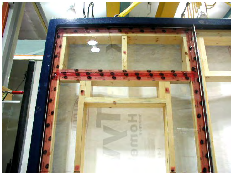
Figure A6-9: Installation and sealing of the clear acrylic sheet in upper part of the Specimen
