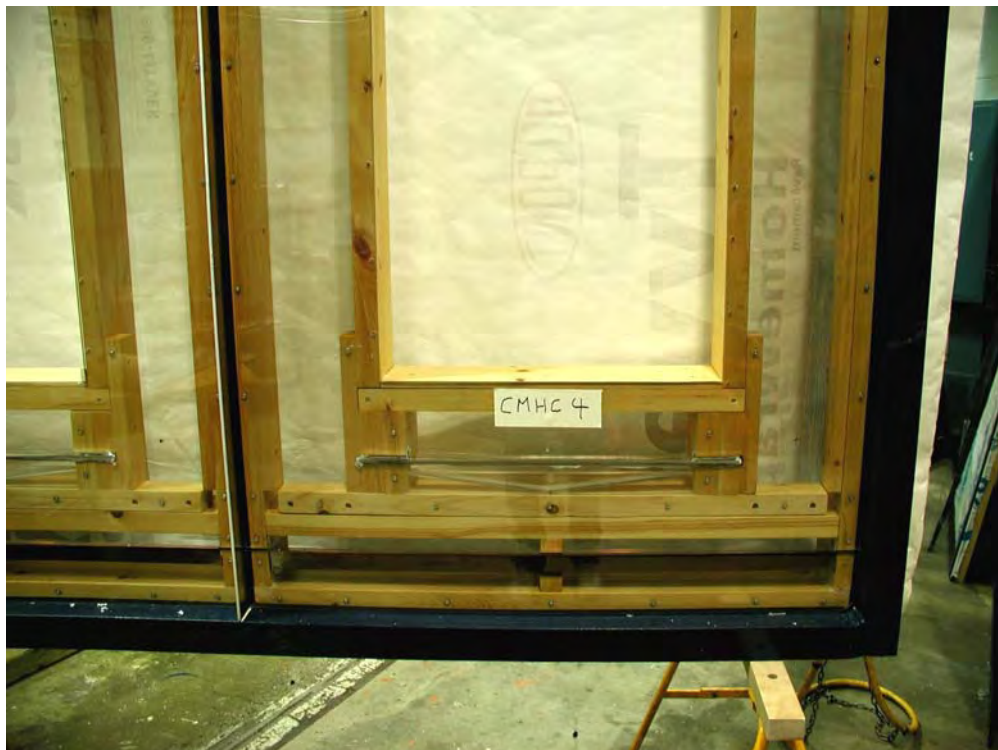
Figure A7-7: Water collection trough under the rough sill in place
