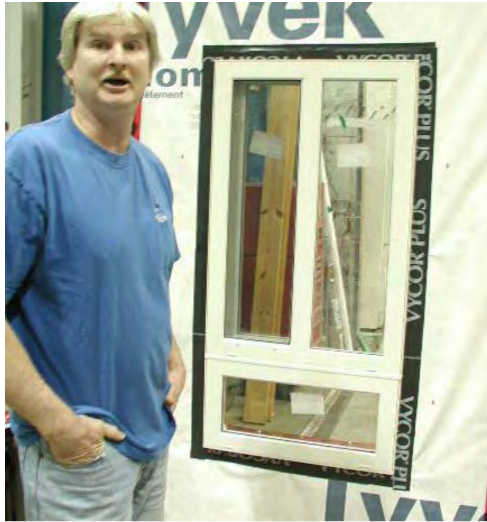
Figure A7-28: Modified Specimen W4 – B-side self-adhered membrane installed at the perimeter of the joint between the WRB membrane and the window flange
