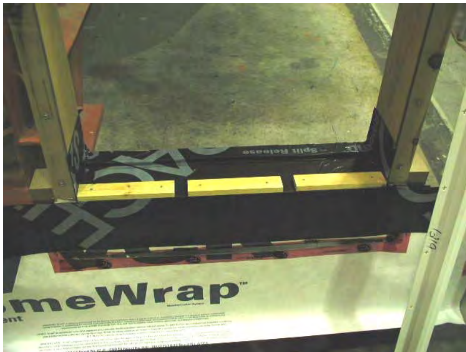
Figure A5-9: Specimen W2 B-side – Placement of wood shims at the sill, over the self-adhesive membrane
