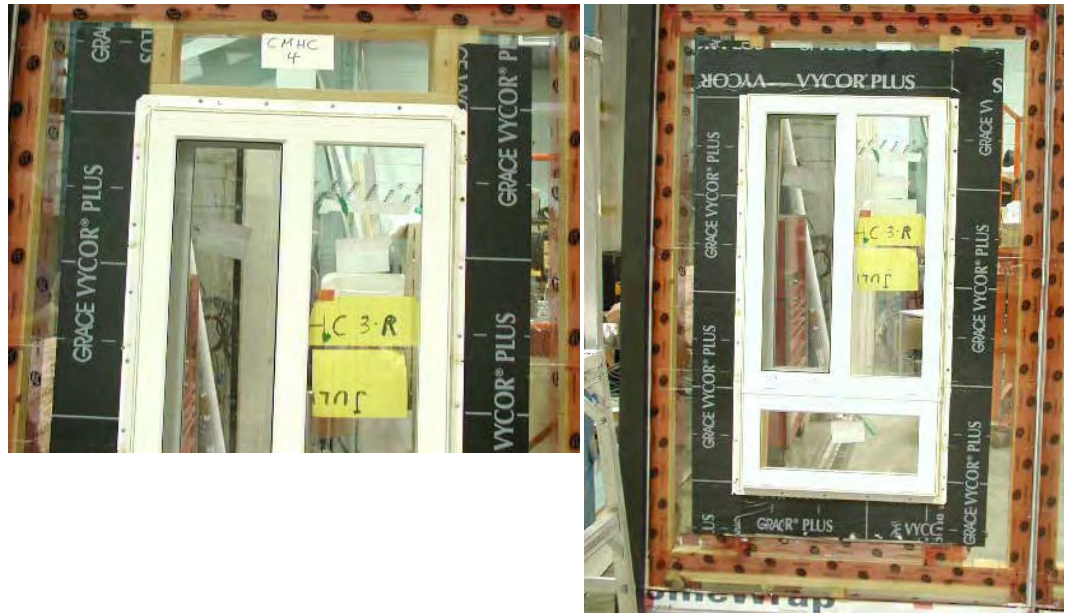
Figure A7-23: Modified Specimen W4 – Installation of self-adhered membrane at the window head over the window flange (the original Specimen did not have that membrane at that location)
