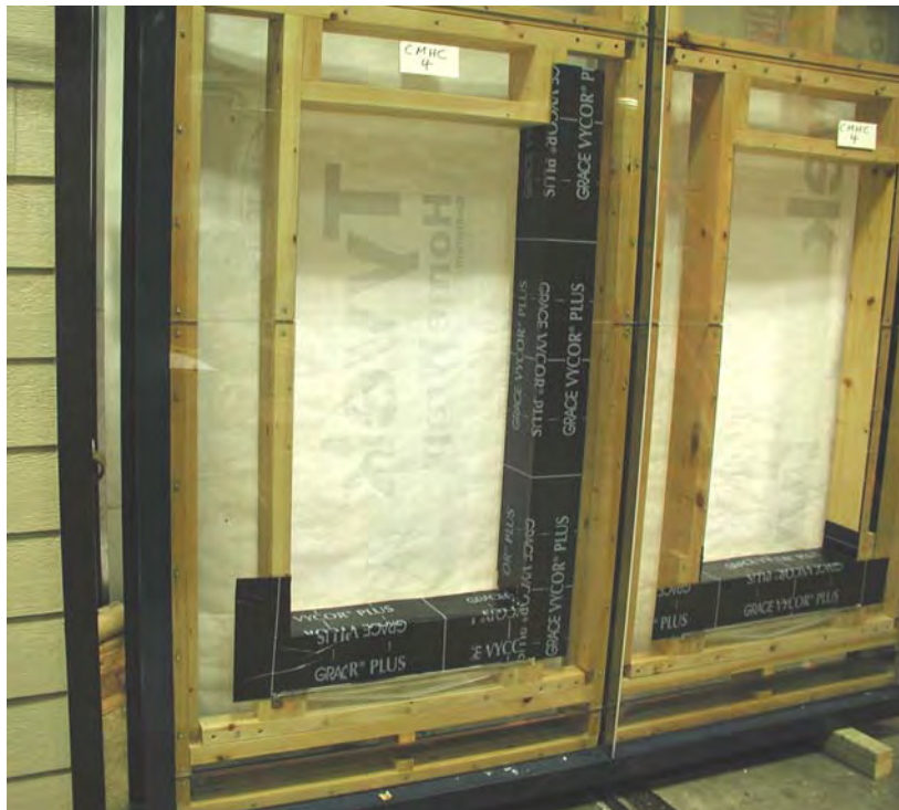
Figure A7-9: Installation of waterproof membrane at the jambs, lapping over the sill membrane
