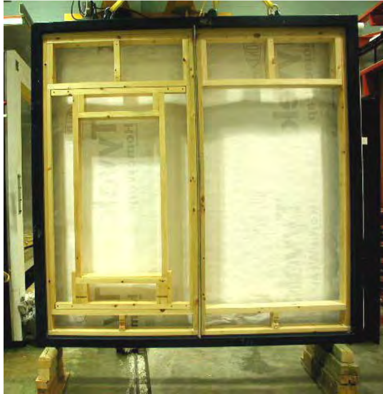
Figure A6-6: Framing for the left hand side of the wall Specimen is completed. Right side is in progress
