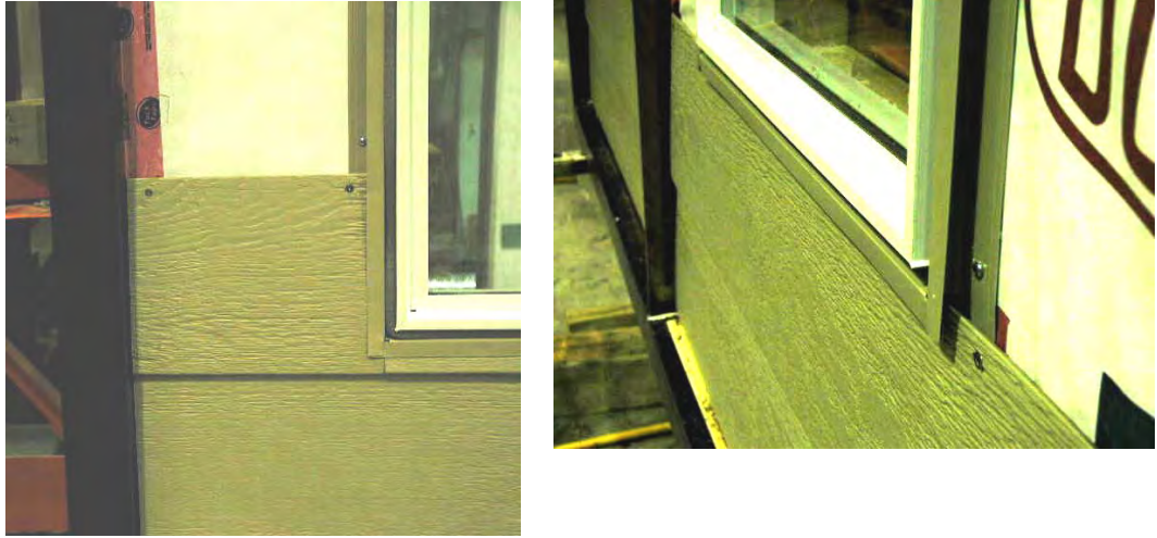
Figure A5-16: Specimen W2 B-side (left side) – Hardboard siding installation with J-trim at sill and jamb (not at the head)
