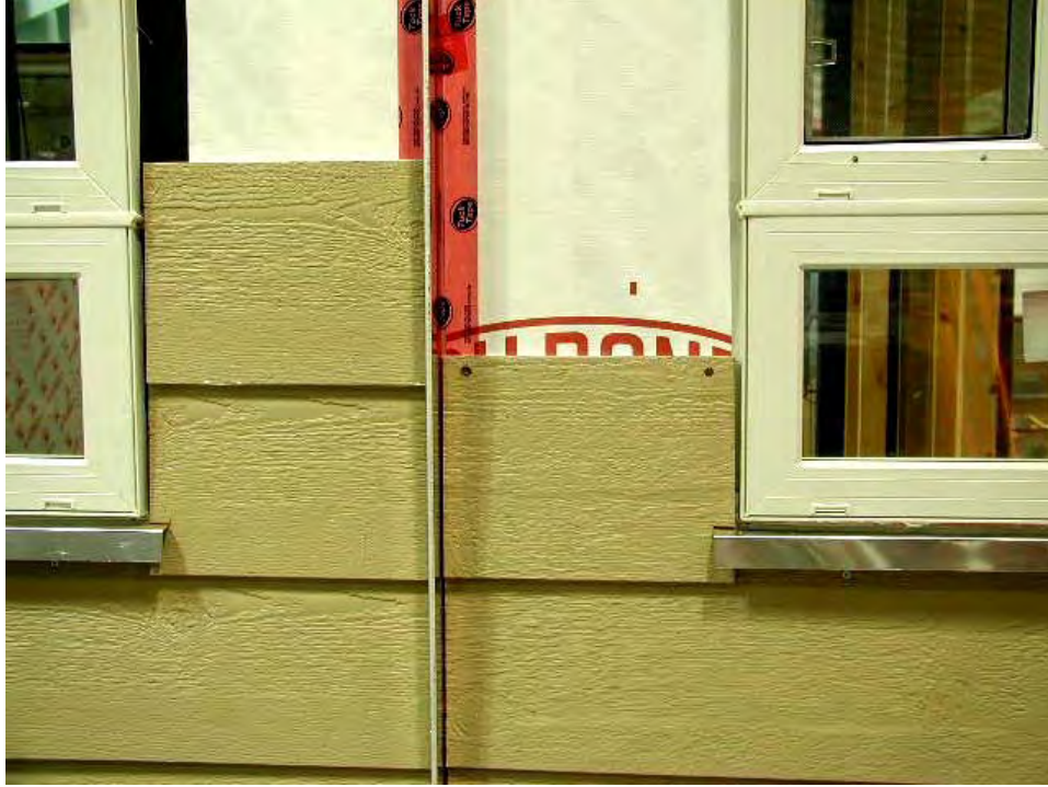
Figure A7-16: Specimen W4 At jambs and head siding was installed 5-mm away from frame of window and spaced 10-mm away from metal drip edge
