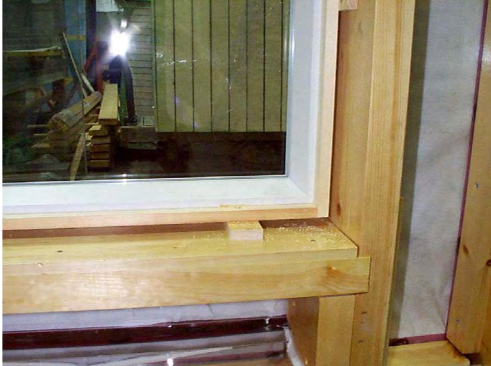
Figure A5-20: Rear view of the Specimen W2 V-side – no membrane protecting the wood members making up the rough opening
