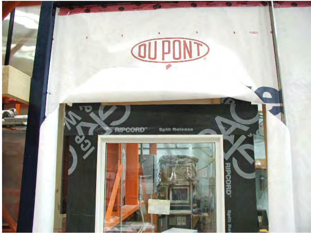
Figure A5-12: Specimen W2 B-side – Placing of the waterproof self-adhesive membrane at the head, over the jamb membrane and over the window flange
