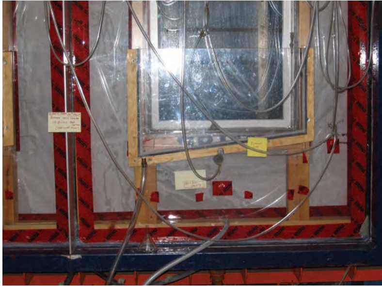
Figure 2-4: Collection trough used for the collection of water penetrating the window
