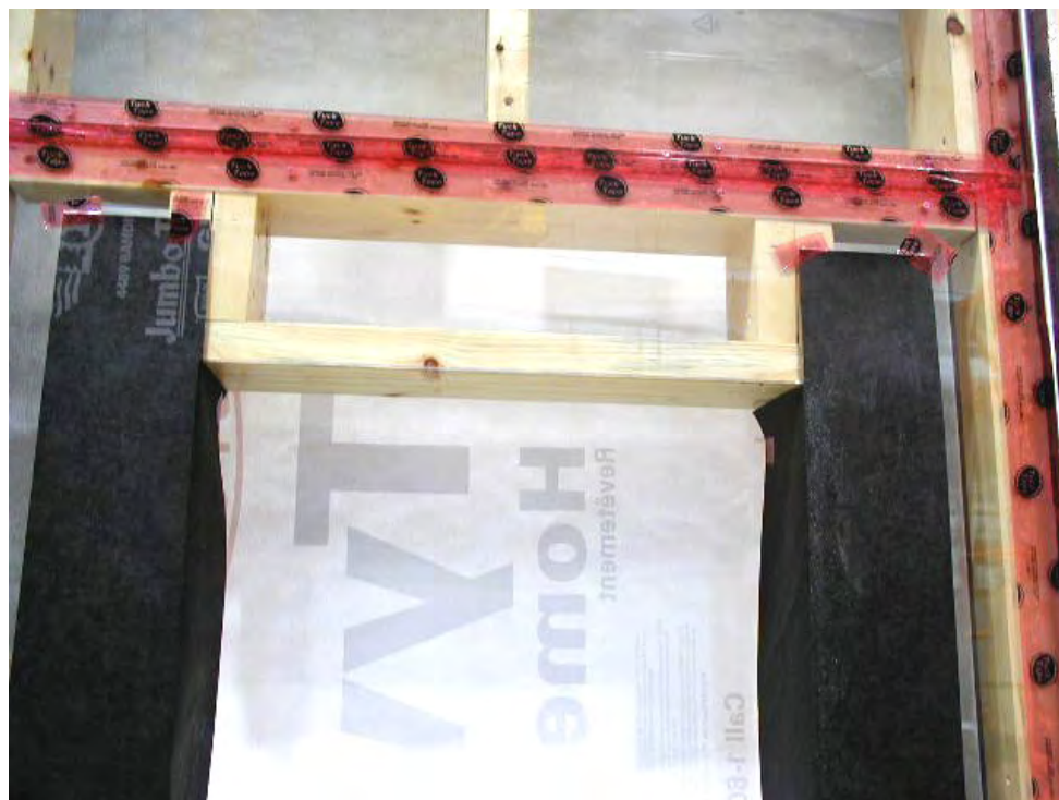
Figure A6-14: Specimen W3 B-side – Installation of strips of building paper at rough jambs
