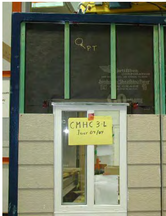
Figure A6-22: Installation of siding on Left and Right sides of Specimen. Siding back-primed and painted (one coat).
