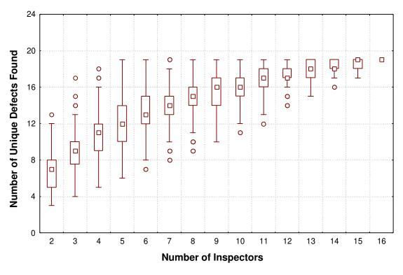
**Figure 1:** Box and whisker plot of unique number of defect against team size from our study. An explanation of box and whisker plots is given in Appendix C.
