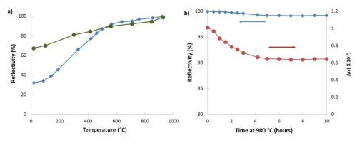
Fig. 6. (a) Isochronal annealing behavior of a low dosage (blue) and high dosage (green) Cgrating; (b) Changes in reflectivity (blue) and index modulation  $\Delta n$  (red) of the low dosage Cgrating under sustained annealing at 900 °C.
