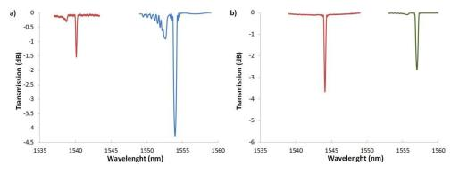
Fig. 5. (a) The initial transmission spectrum of the high-dosage B-grating with a room temperature resonance at 1540 nm (red trace) and its spectrum at 1000 °C after several hours of annealing at 1000 °C (blue trace); (b) The transmission spectra of the initial room temperature low dosage B-grating (red trace) and its spectrum at 1000 °C after annealing at 1000 °C (green trace).
