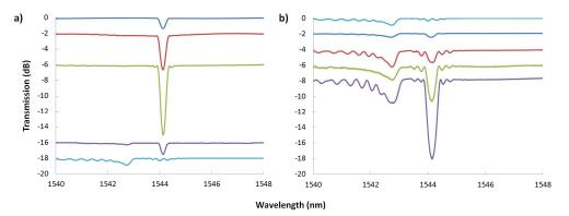
Fig. 1. Evolution of the transmission spectra of (a) type I-like grating and (b) type II grating as a function of laser exposure. Transmission spectral traces are offset vertically for ease of viewing and correspond to increments of 15 laser pulses per trace.
