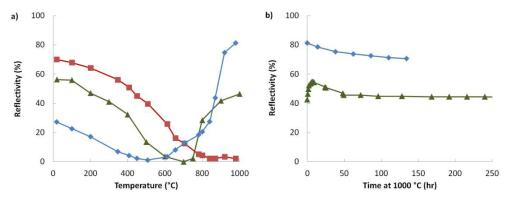
Fig. 4. (a) Grating reflectivity variation as a function of isochronal annealing temperature. Red trace is a standard type I grating, blue trace is the high dosage B-grating, the green trace is the low dosage B-grating; (b) denotes the stabilization of low dosage (green) and high dosage (blue) B-gratings when annealed at 1000 °C.
