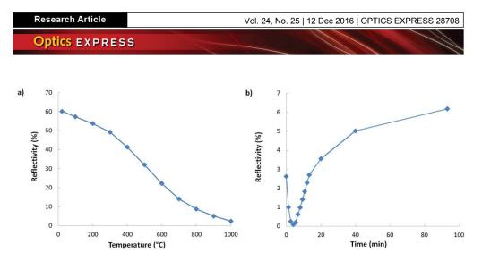
Fig. 3. (a) Change in reflectivity of the stage A-grating during isochronal annealing; (b) evolution of a thermally stable grating as a function of time at 1000 °C.
