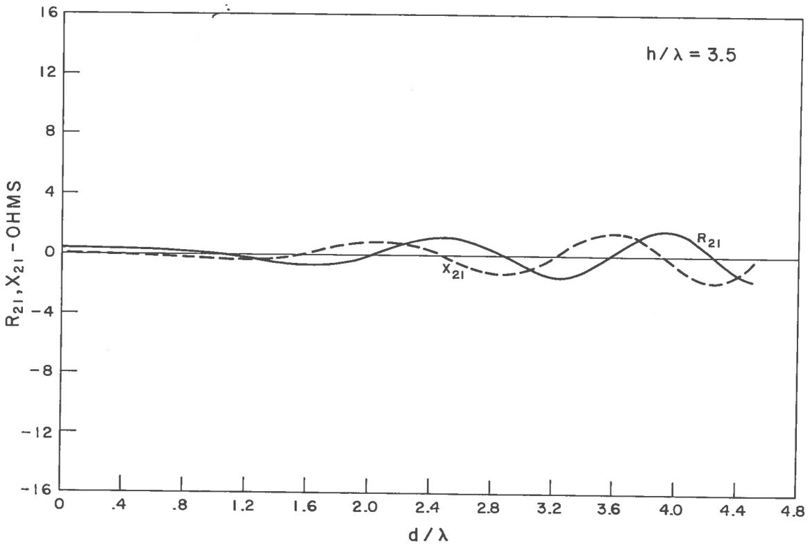
Fig. 9 Mutual impedance of two staggered parallel half-wave dipoles for  $h/\lambda = 3.5$
