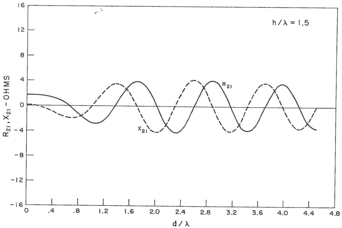
Fig. 5 Mutual impedance of two staggered parallel half-wave dipoles for  $h/\lambda = 1.5$
