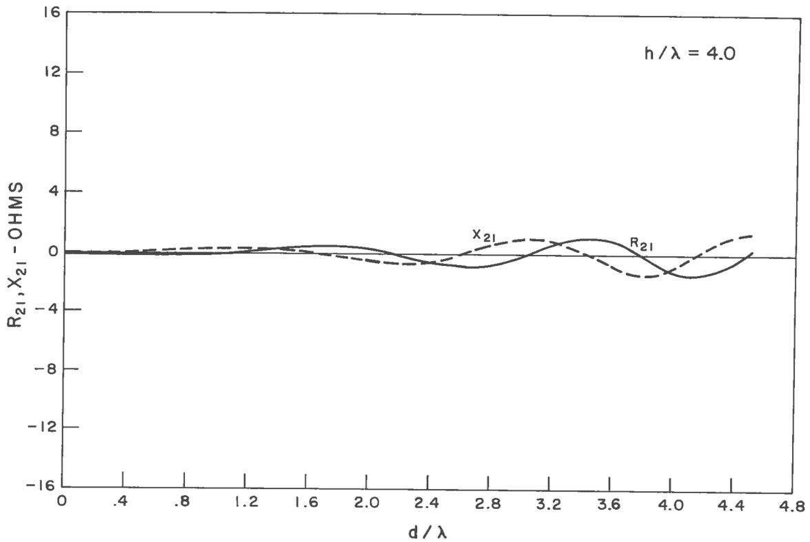
Fig. 10 Mutual impedance of two staggered parallel half-wave dipoles for  $h/\lambda = 4$
