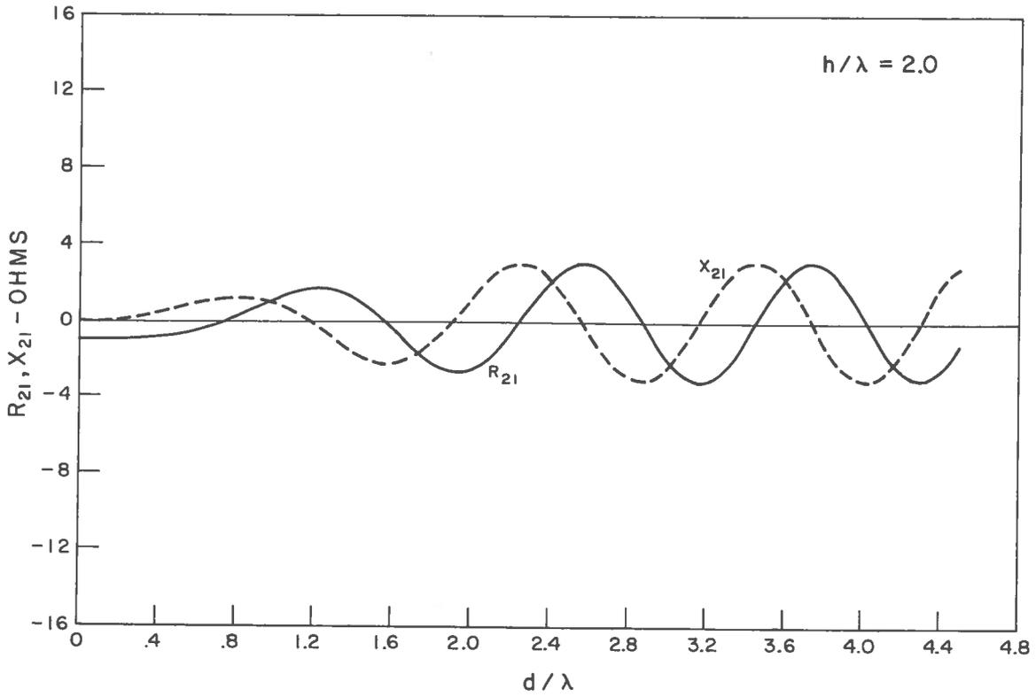
Fig. 6 Mutual impedance of two staggered parallel half-wave dipoles for  $h/\lambda = 2$
