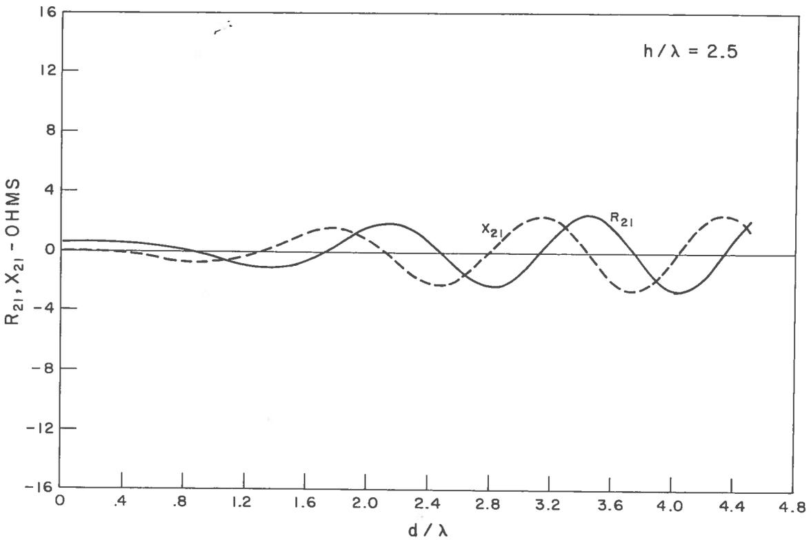
Fig. 7 Mutual impedance of two staggered parallel half-wave dipoles for  $h/\lambda = 2.5$
