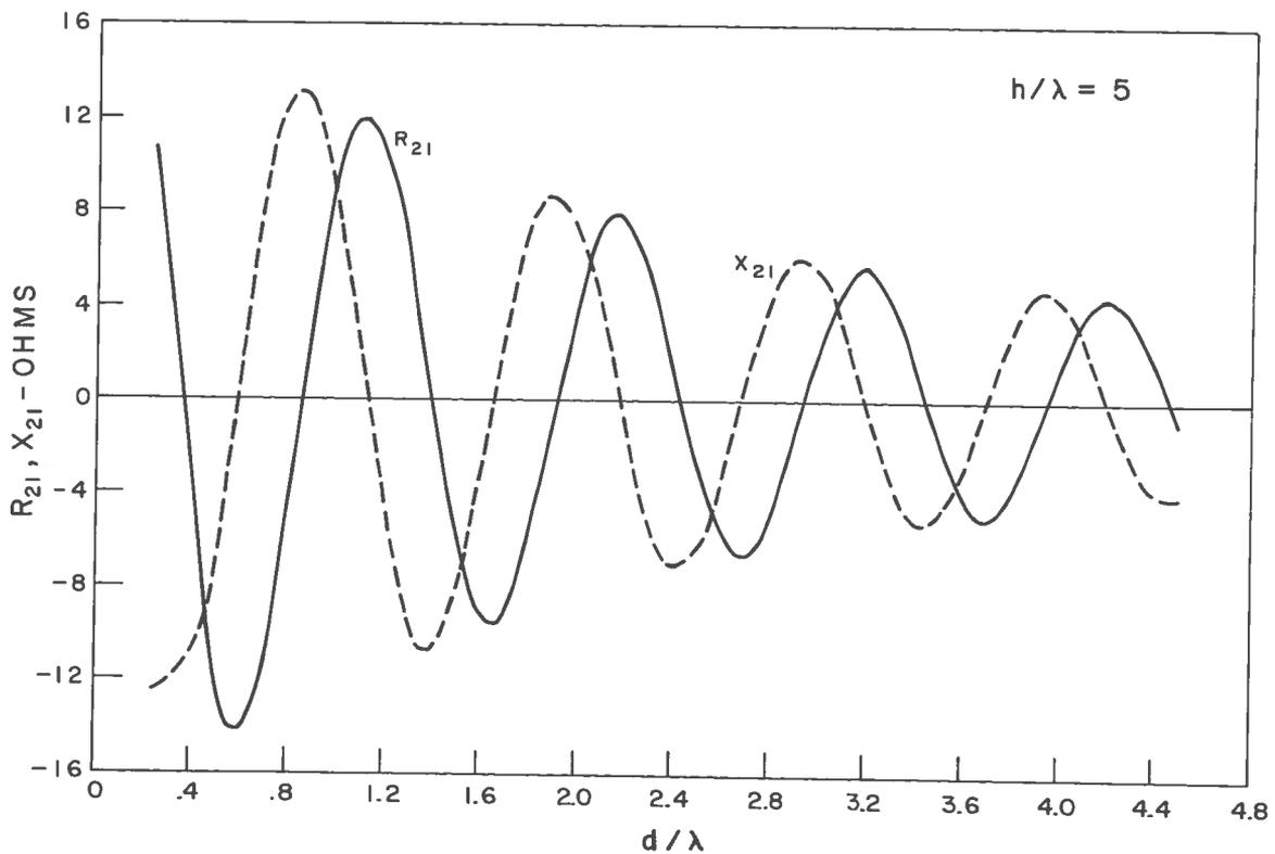
Fig. 3 Mutual impedance of two staggered parallel half-wave dipoles for  $h/\lambda = 0.5$
