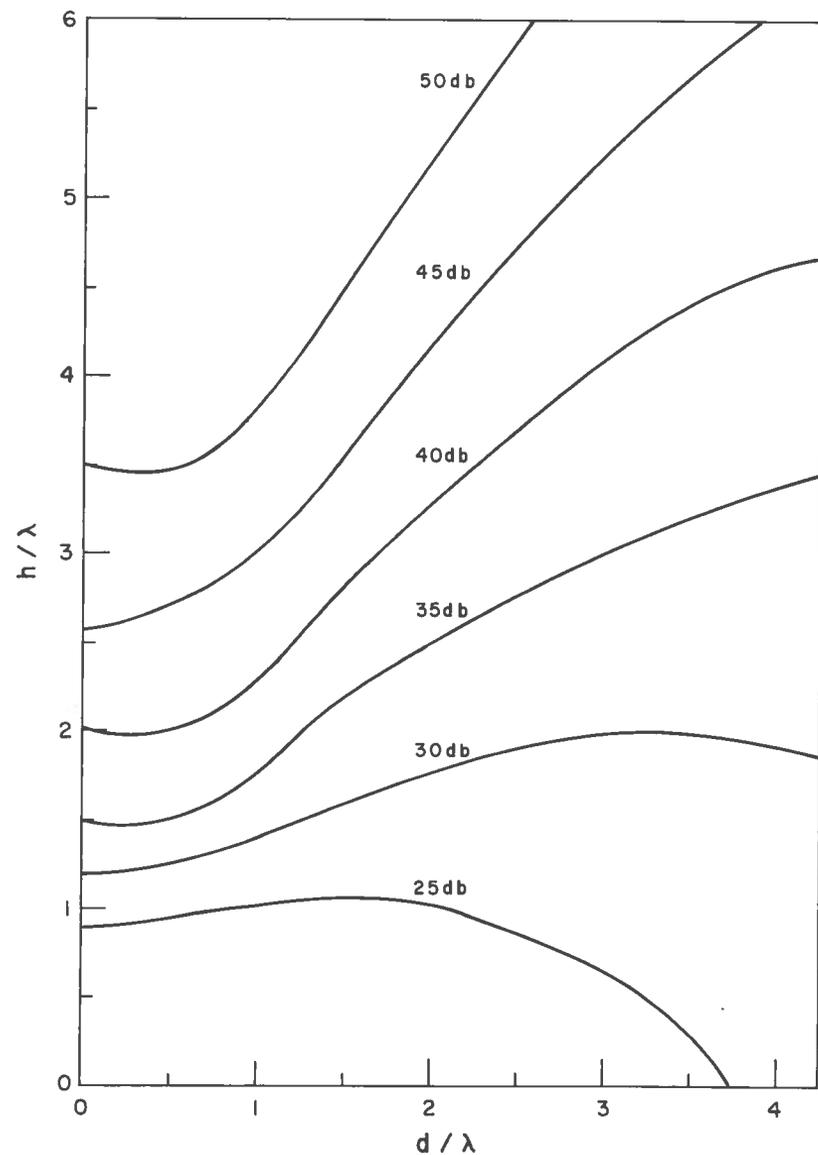
Fig. 13 Constant isolation contours for two staggered parallel half-wave dipoles
