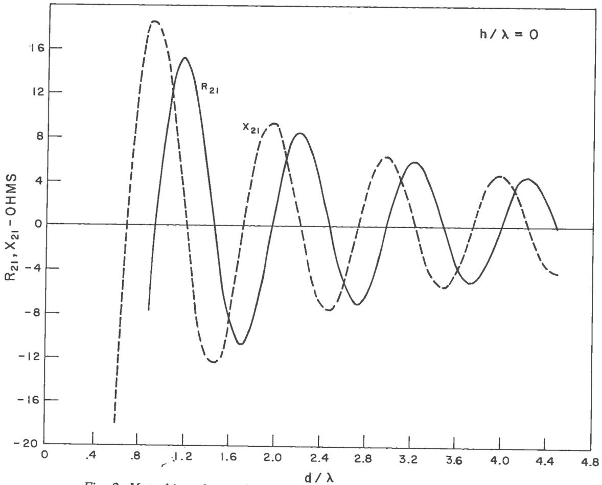
Fig. 2 Mutual impedance of two staggered parallel half-wave dipoles for  $h/\lambda = 0$
