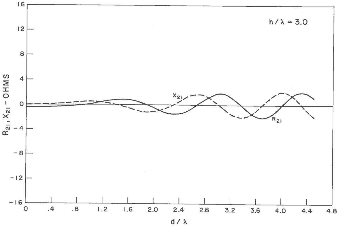
Fig. 8 Mutual impedance of two staggered parallel half-wave dipoles for  $h/\lambda = 3$
