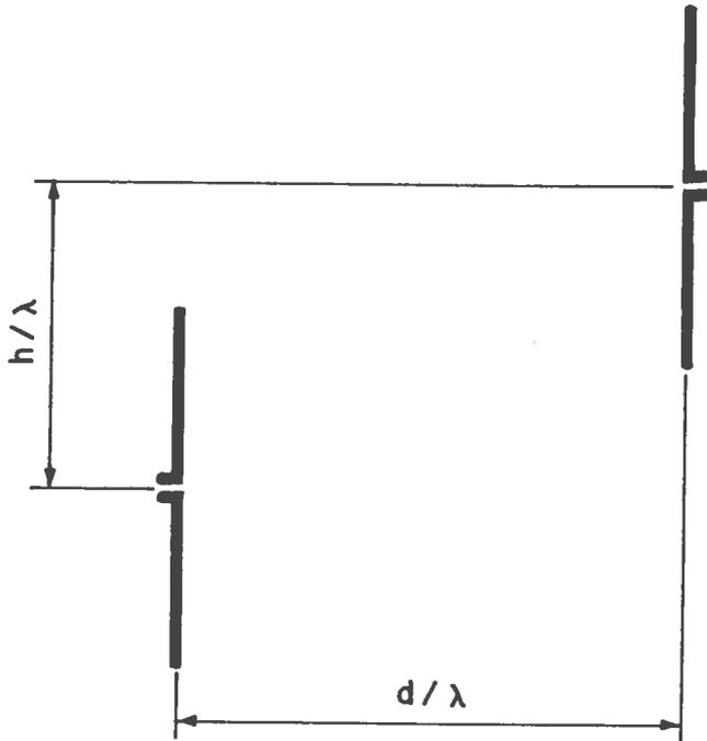
Fig. 1 Antenna geometry used in calculations.
