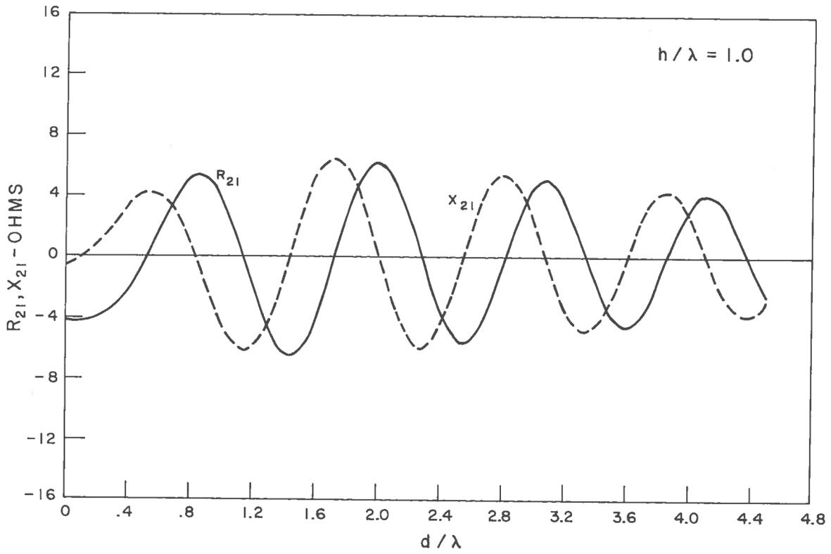
Fig. 4 Mutual impedance of two staggered parallel half-wave dipoles for  $h/\lambda = 1$
