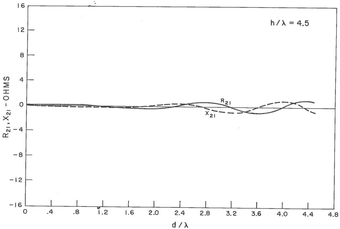
Fig. 11 Mutual impedance of two staggered parallel half-wave dipoles for  $h/\lambda = 4.5$
