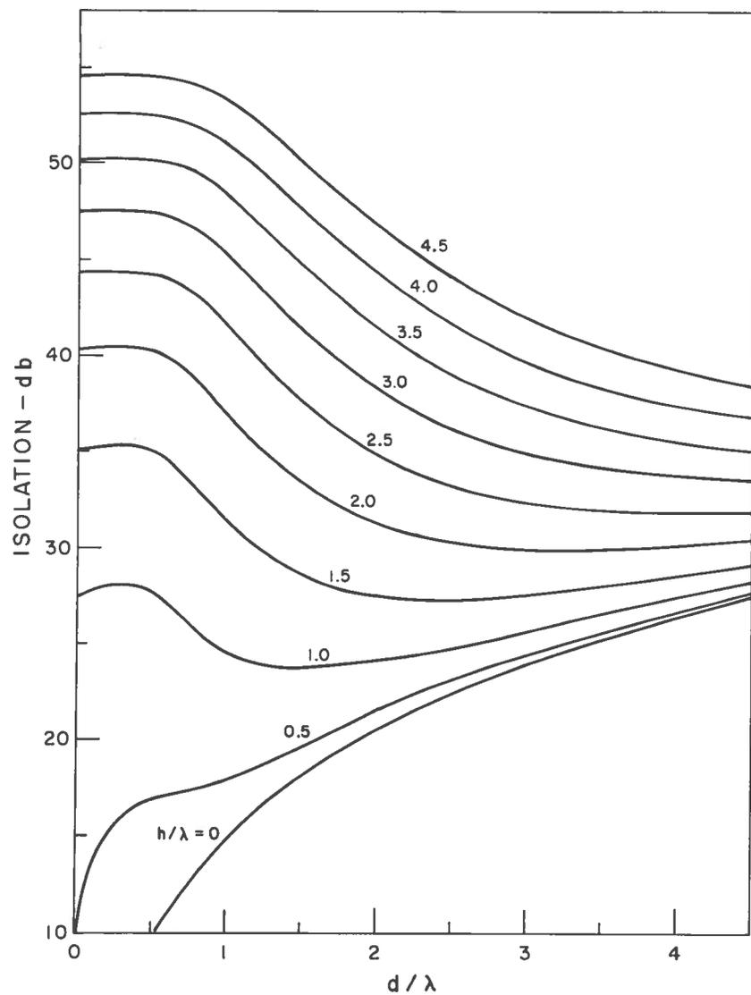
Fig. 12 Isolation of two staggered parallel half-wave dipoles as a function of antenna spacing
