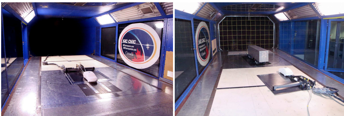
Figure 2.1: Left: view from upstream of vehicle alone (case VEH), Right: view from downstream of vehicle and HDV model.
