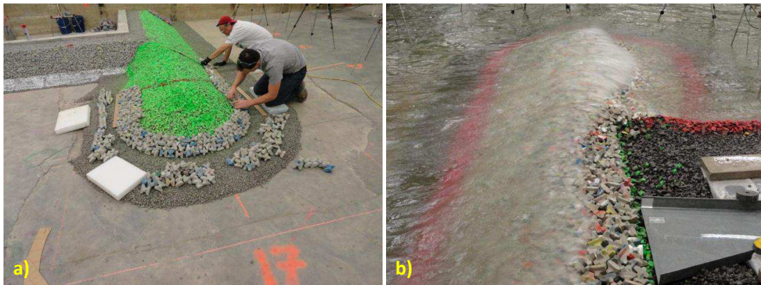
Figure 2. Stability assessment for the north and stub breakwaters.
