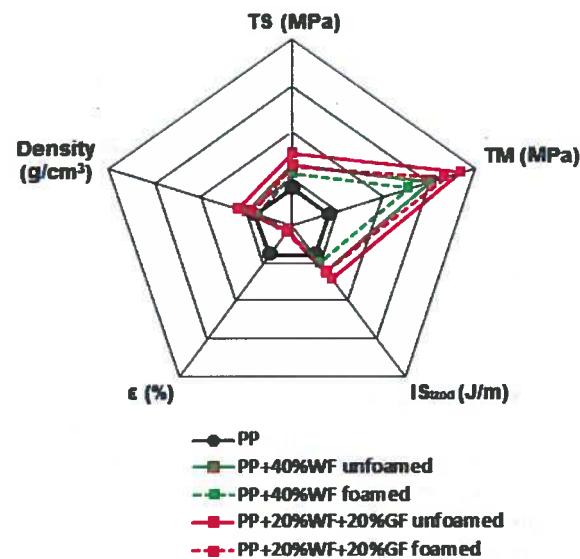
Figure 4. Properties comparison for virgin PP, unfoamed and foamed PP/40 wt.%WF, and unfoamed and foamed PP/20 wt.% WF/20 wt.% GF hybrid.
