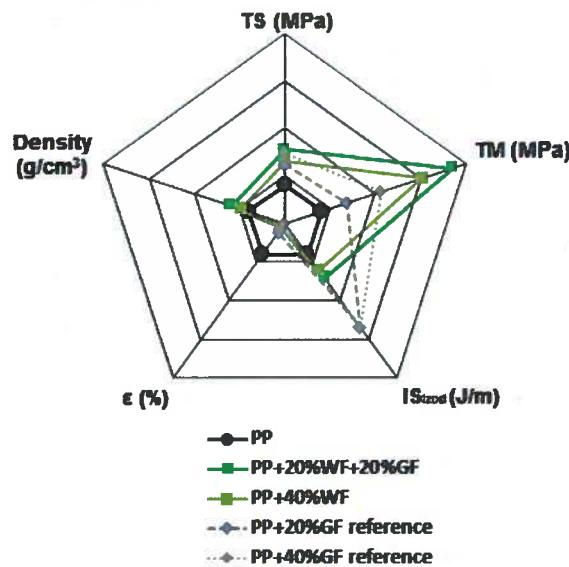
Figure 3. Properties comparison for different PP-based biomaterials.
