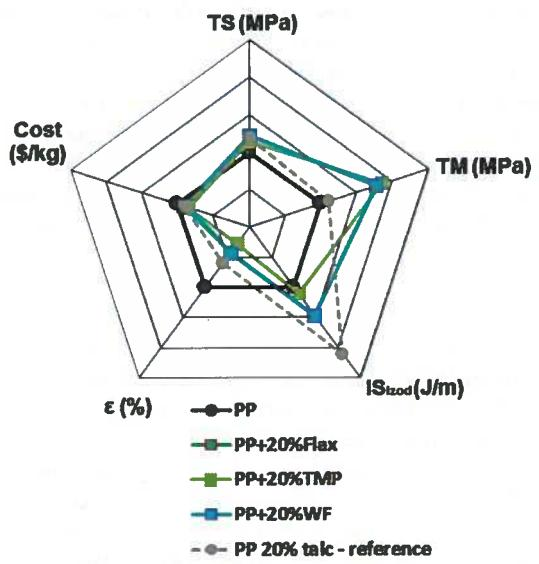
Figure 2. Properties comparison for PP, PP-based biocomposites and PP reference.
