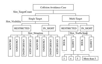
Fig. 3 The hierarchical indexing tree of a case base for collision avoidance
