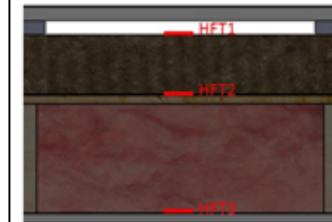
Figure 4. Horizontal cross-section through mineral fibre wall assembly showing locations of Heat Flux Transducers, HFTs (Wall 3)
