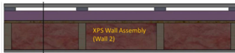
Figure 1. Schematic of three residential 38 mm x 140 mm (2 x 6 in.) wood-frame wall test specimens installed side-by-side in the FEWF
