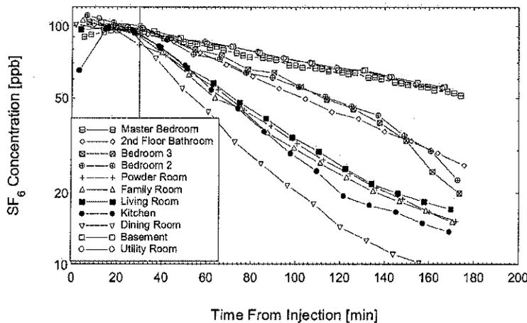
Figure 8b Simultaneous room-by-room decay measurements for configuration B at  $+11^{\circ}\text{C}$ . Local exhaust system—vents open.
