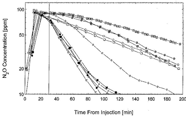
Figure 8a Simultaneous room-by-room decay measurements for configuration B at  $-24^{\circ}\text{C}$ . Local exhaust system—vents open.
