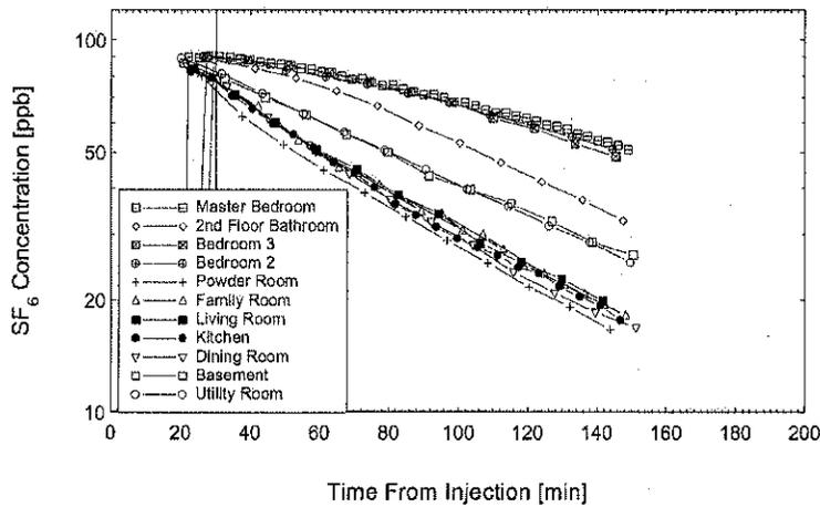
Figure 9a Simultaneous room-by-room decay measurements for configuration C at  $-19^{\circ}\text{C}$ . Partially distributed exhaust system—vent sealed.
