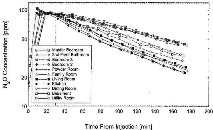
Figure 9b Simultaneous room-by-room decay measurements for configuration C at  $+11^{\circ}\text{C}$ . Partially distributed exhaust system—vent sealed.
