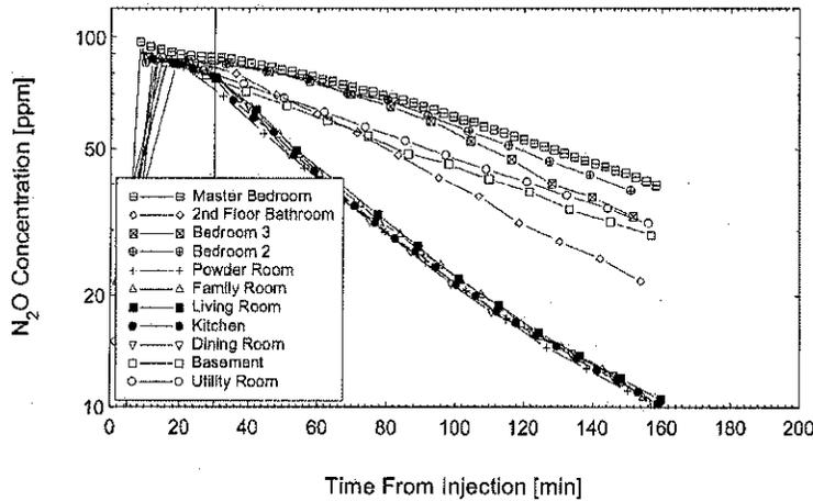
**Figure 10a** Simultaneous room-by-room decay measurements for configuration D at  $-23^{\circ}\text{C}$ . Partially distributed exhaust system—vent open.
