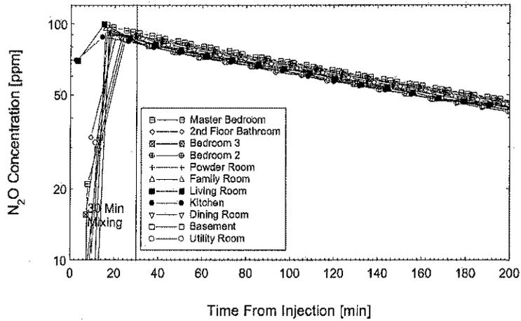
Figure 6 Simultaneous room-by-room decay measurements for configuration G at  $-19^{\circ}\text{C}$ . Reference case—windows and vents sealed, fans off, furnace fan on.
