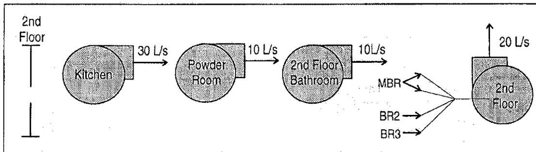
Figure 3 Schematic illustration of partially distributed exhaust strategy—configuration C, vent closed; configuration D, vent open.
