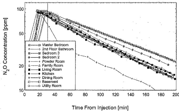
**Figure 11a** Simultaneous room-by-room decay measurements for configuration E at  $-14^{\circ}\text{C}$ . Minimal ducted supply system with local exhaust system—no vents.
