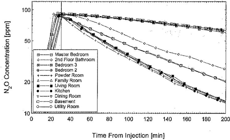
Figure 7a Simultaneous room-by-room decay measurements for configuration A at  $-23^{\circ}\text{C}$ . Local exhaust system—vents sealed.
