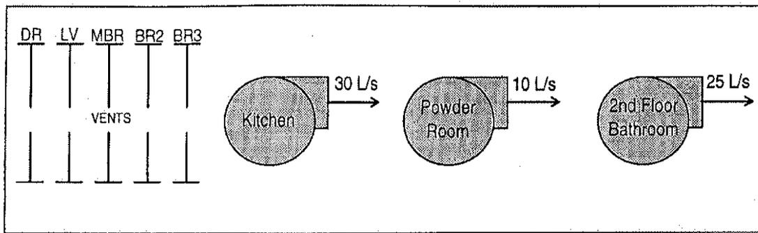
Figure 2 Schematic illustration of local exhaust fan strategy—configuration A has vents closed, configuration B has vents open.
