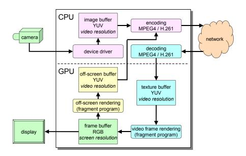
**Figure 3.** Video coding and decoding data paths, using GPU for conversion and resizing. Some intermediate storage is omitted for clarity.
