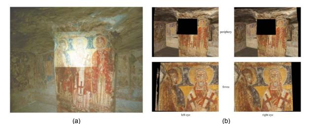
**Figure 4.** Foveated stereoscopic display. (a) photograph of the screen (only one eye's view is shown for clarity); (b) the four original images composing (a).
