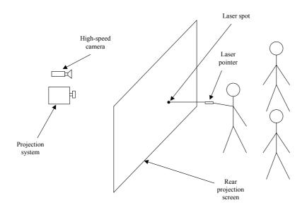
Figure 5. Laser-based interaction with wall screen.
