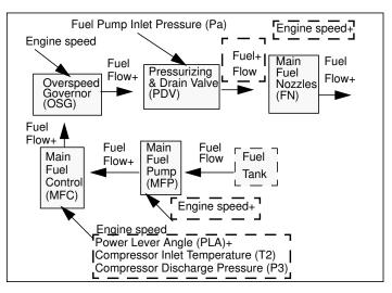
Fig. 2. Main Fuel System model extracted by DR
