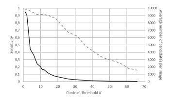
**Fig. 3.** Sensitivity (dashed line) and average number of candidates per image (solid line) as functions of the contrast threshold K.
