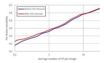
**Fig. 4**. FROC curves computed on the test images, before and after OD removal.
