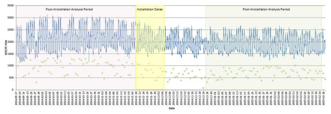
Figure 3. Seven months of energy data for the sub-metered circuit with 48 LED luminaires. The blue line shows 15-minute total energy use data (circuit included other loads), the green markers show daily rise metric used for statistical analysis. Date ranges used in statistical analysis are shown (note, only normal weekday values in these ranges were used).
