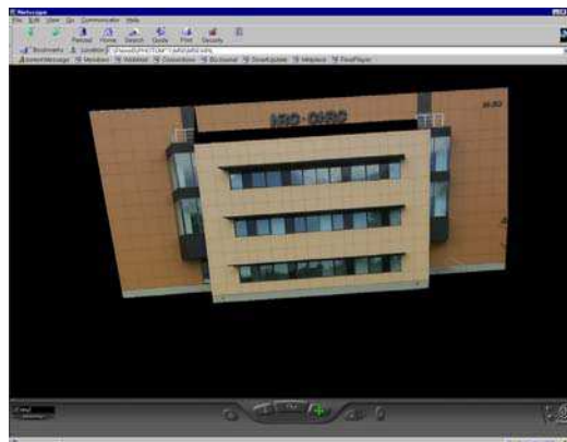
Figure 12: 3D textured model of NRC building created by ShapeCapture.
