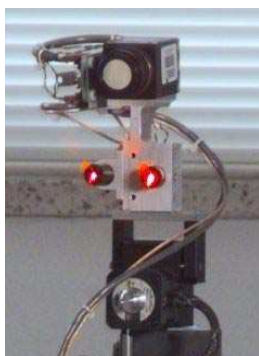
Figure 6. Photograph of the 3-D Range Sensor and its Pan-Tilt Unit
