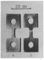
Fig. 1 Tensile specimens of Al<sub>s</sub>,Ti<sub>25</sub>Mn. alloy (a) before and (b) after test
