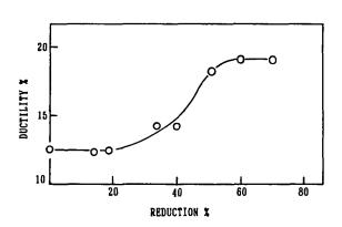
Fig. 3 Room temperature compressive ductility of hot-pressed and annealed AlerTizeMne alloy as a function of reduction
