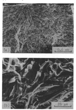
Fig. 6 SEM fractographs of tensile tested specimen of Als7Ti25Mns alloy
