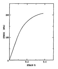
Fig. 5 Typical tensile stress-strain curve of the AlerTi25Mns alloy, 70% hot-pressed and 1273K/2h annealed
