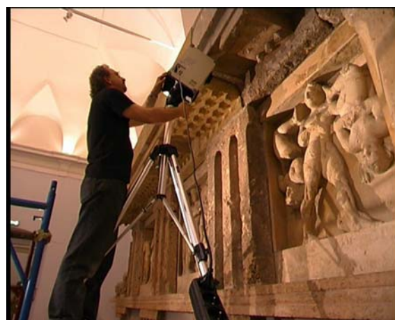
Fig. 4 - Practical considerations when using a 3D scanner: mirror used to reach hidden 3D surfaces.
