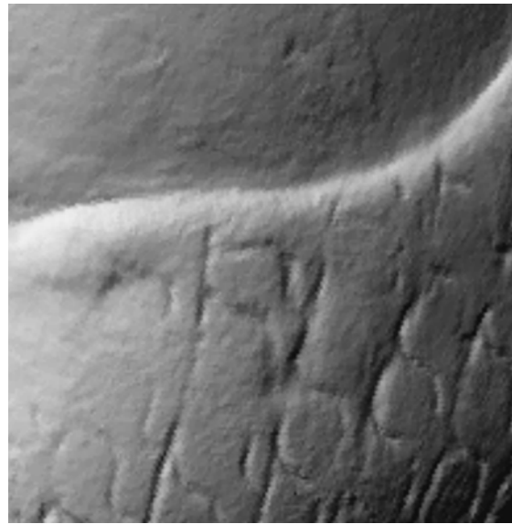
Fig. 10 - Close-ups (~ 25 mm × 25mm), a) shaded view created from the 3D data acquired with a Minolta 900 (tele-lens), b) shaded view created from the 3D data acquired with a ShapeGrabber SG-102 head mounted on a translation stage.
