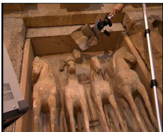
Fig. 4 - Practical considerations when using a 3D scanner: mirror used to reach hidden 3D surfaces.
