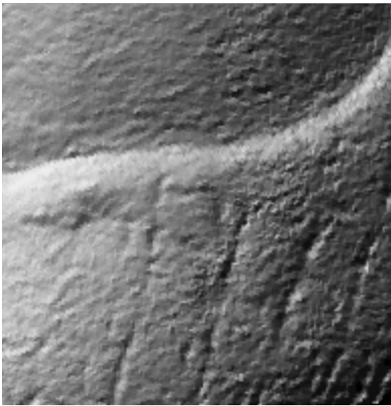
Fig. 10 - Close-ups (~ 25 mm × 25mm), a) shaded view created from the 3D data acquired with a Minolta 900 (tele-lens), b) shaded view created from the 3D data acquired with a ShapeGrabber SG-102 head mounted on a translation stage.
