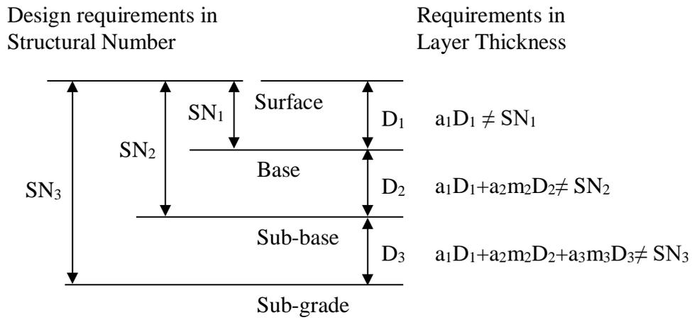
Fig 1. The concept of layer analysis
