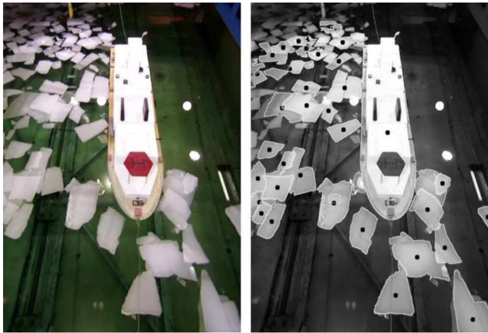
Figure 4: Accurate Image Segmentation with Touching Pieces and Inconsistent Lighting (Gash and Millan, 2012)
