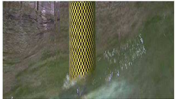
Photo 2: Testing of a single shaft GBS with high waves is in progress
