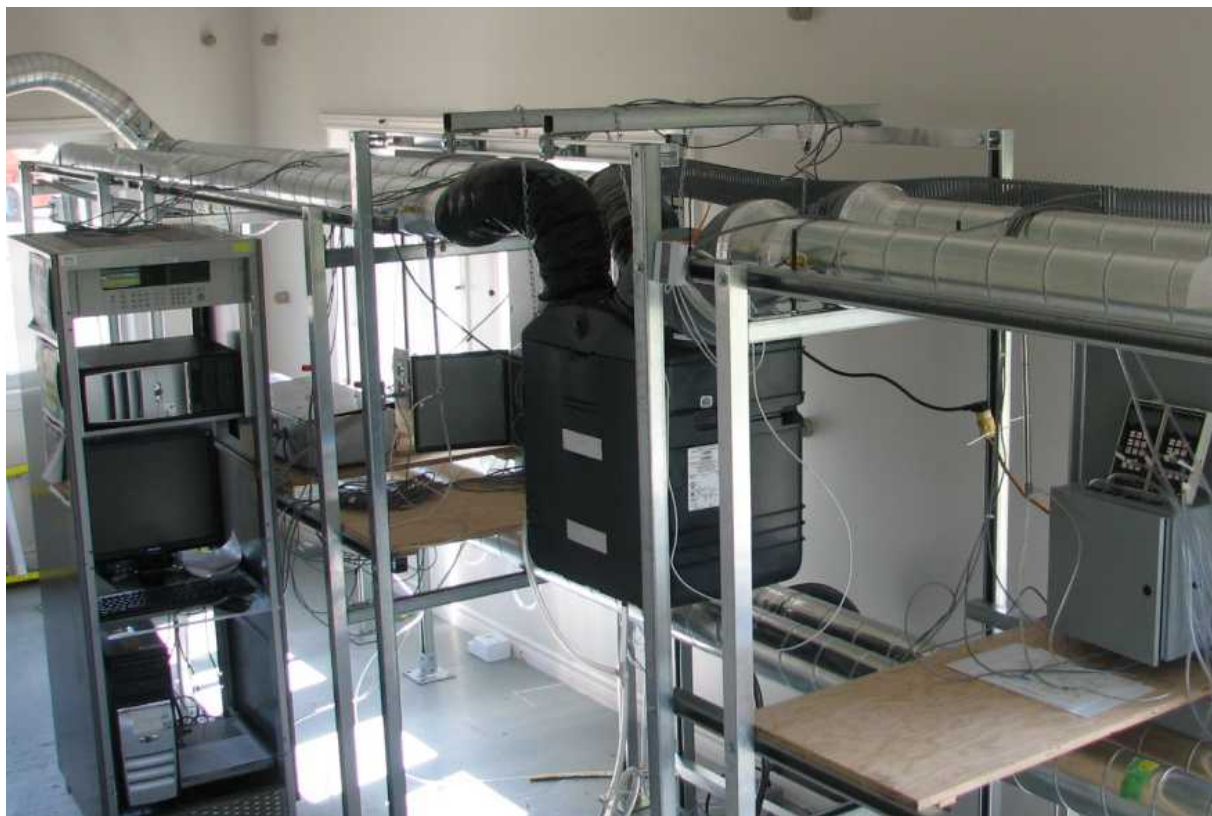
Figure 7-3: Example of an actual installation of the HRV/ERV system test rig.
