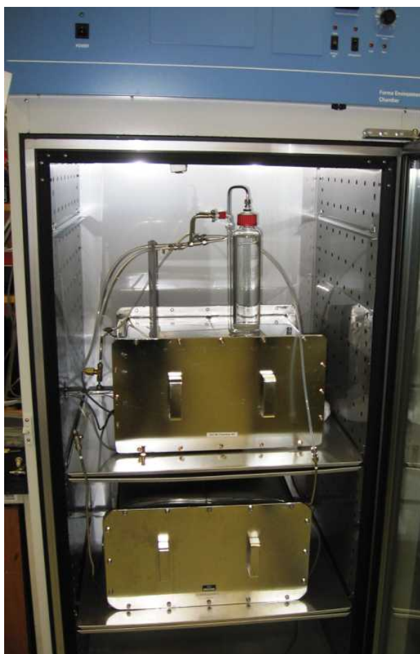
Figure 7-4: Small chamber system for headspace analysis of component emissions.
