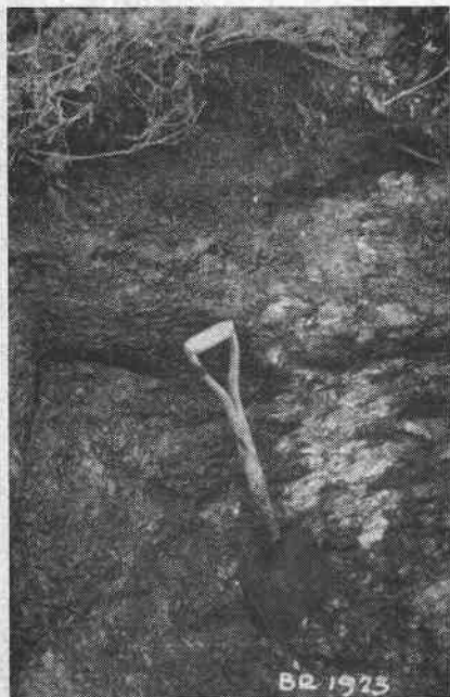
Fig. 4. Test pit excavated by pick and shovel in fine-grained soil. Note occurrence of ice to right of shovel and also slumping and thawing of material on left side of pit.
