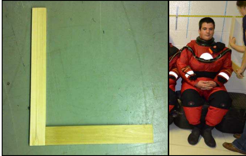
Figure 2.9: Wooden carpenter's square (left), and the square being used to obtain group anthropometric measurements (right).
