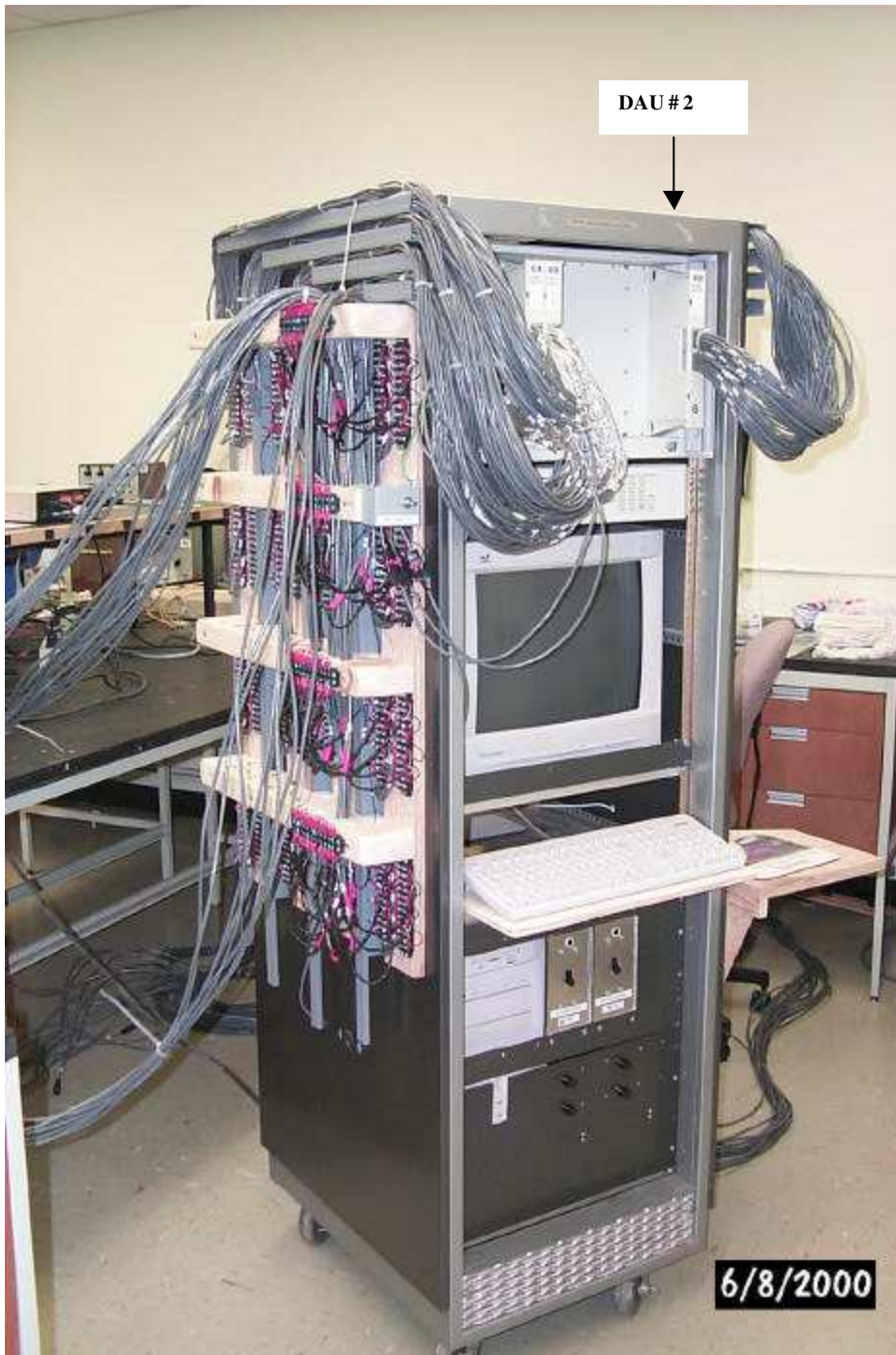
Figure 33 Connection of the probe to Data Acquisition Unit # 2(DAU)
