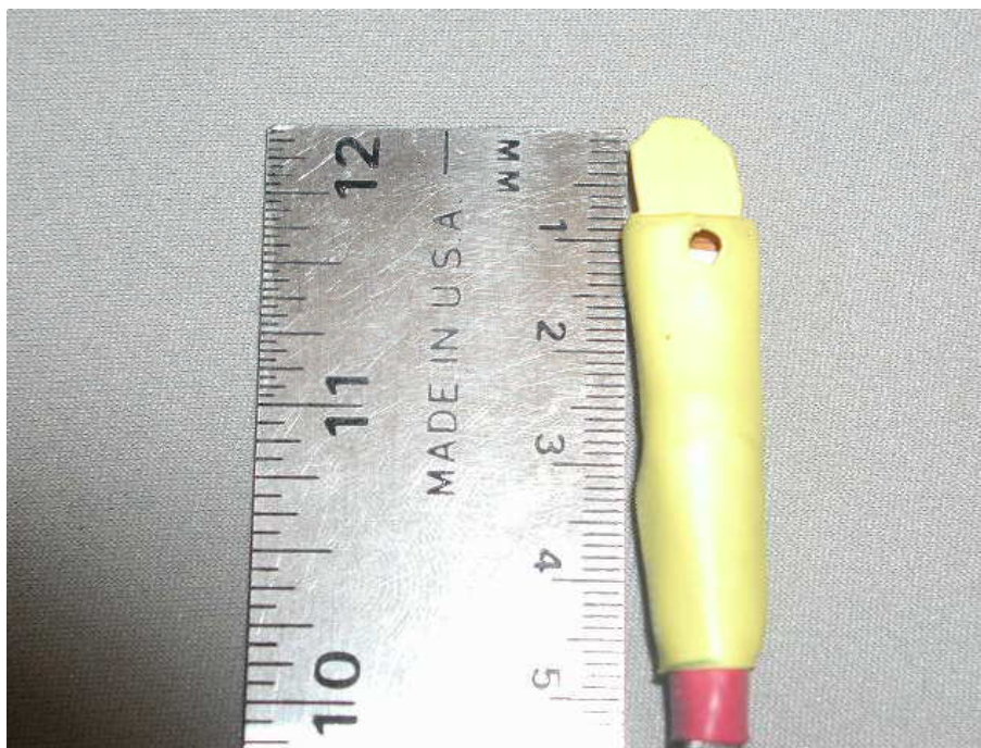
Figure 30 Close-up view of the shroud in place over the tip of the probe
