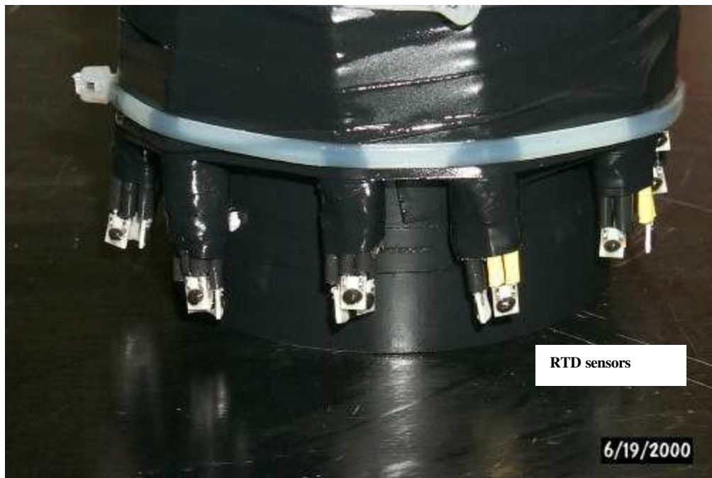
Figure 9 Close-up of RTDs grouped on an insulated aluminum cylinder
