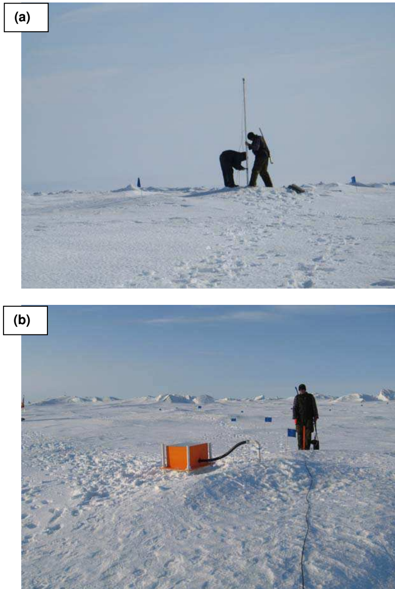
Figure 18 Temperature chain 'A' on Floe R02 (a) installing temperature chain between flags 25 and 26 on Transect 5 and (b) completed installation with elevated orange box housing the data acquisition system, GPS and Iridium phone communications.
