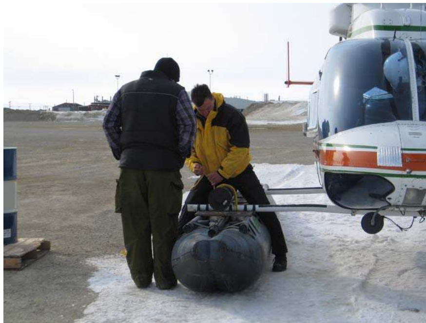
Figure 3 Transporting temperature chain to Floe R02. The five 2 m lengths of temperature chain were sealed in a black ABS tube and securely strapped to the helicopter skids.
