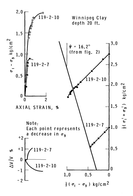
FIGURE 6 CONSOLIDATED DRAINED TRIAXIAL TEST RESULTS LATERAL STRESS DECREASED IN STAGES
