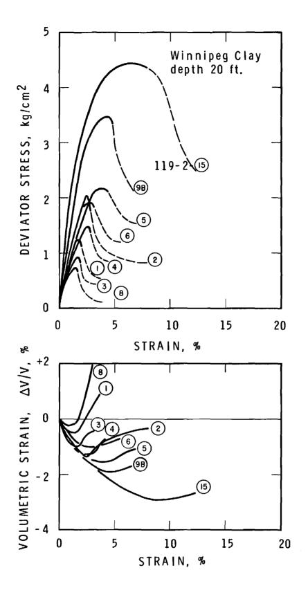
FIGURE 1 CONSOLIDATED DRAINED TRIAXIAL TEST RESULTS - AXIAL STRESS INCREASING
