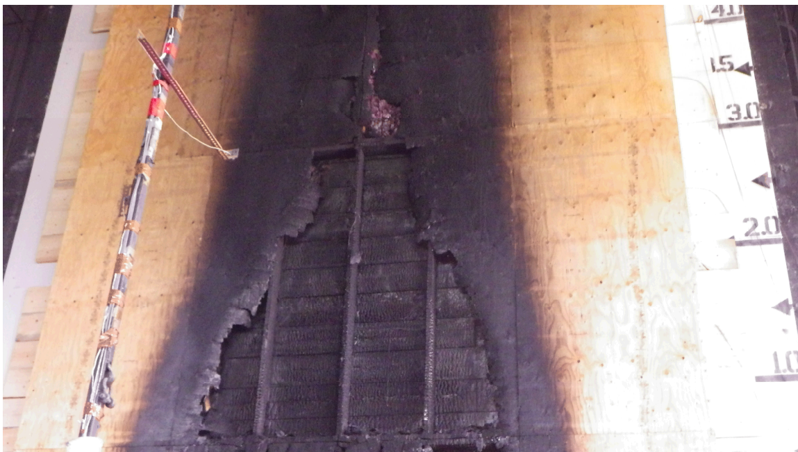
Figure 13. Wall Sample after Fire Exposure.
