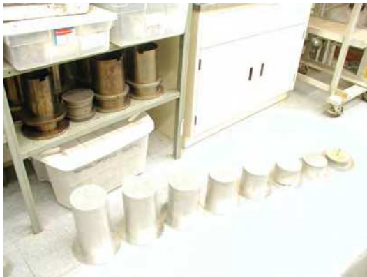
Figure 9. Cylindrical adapters used for compaction of granular specimens
