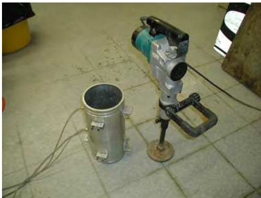
Figure 8. Split mold and vibrator for preparation of granular specimens
