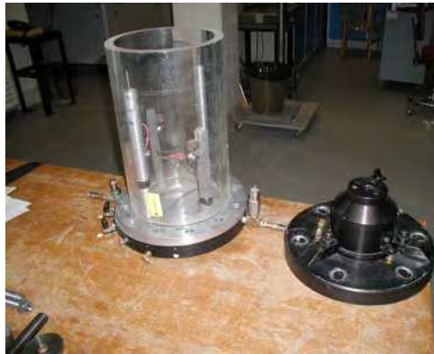
Figure 2. Triaxial Pressure Chamber (152.4 mm; 6 in.-cell configuration)
