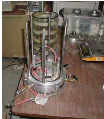
Figure 3. Triaxial pressure chamber (76.2 mm; 3 in.- cell configuration)
