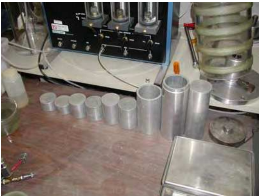
Figure 12. Equipment for preparation of cohesive specimens
