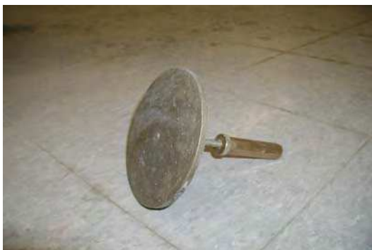
Figure 10. 152.4 mm (6 in.)-Diameter spacer
