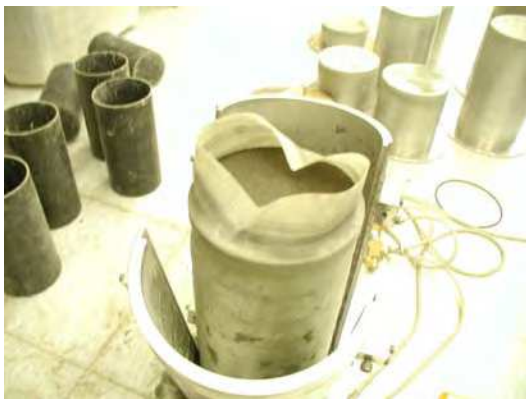
Figure 28. Granular sample preparation step #9
