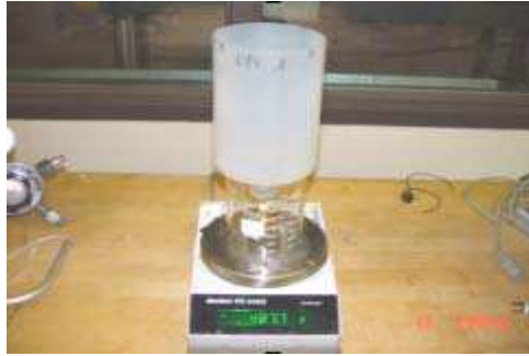
Figure 2a. Weigh scale and foam expansion and drain apparatus
