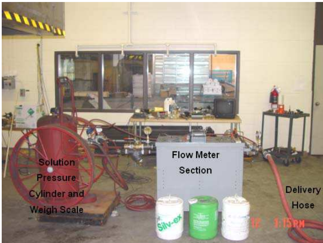
Figure 2b. Foam delivery apparatus.
