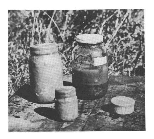
Fig. 7 - The various types of soil samples are shown ready for shipment. The sealed tin and jar in front were used for moisture and organic contents. The sealed jar on the left contains a unit weight sample while the unsealed glass jar was used for specific gravity, grain size distribution, and Atterberg limit tests. Note large volume of water in unsealed glass jar.
