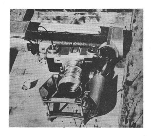
Fig. 6 - The camera assembly that was used to photograph frozen cores. The camera is a Contax with four supplementary lenses equivalent to Portra 10. The mirrored light source is a Powell Repeater Flash with a 1/1500 sec. light duration and the lens opening used was f22. The unit is the personal property of Dr. T. Hunt, National Health and Welfare Department.
