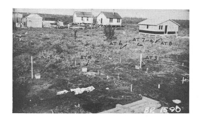
Fig. 3 Thermocouple installations at the proposed teacherage site. The organic cover averages 12 inches and the area has been cleared of shoulder-high alder willow thicket. Thermocouple installations AT3, 4, and 5 are under a typical floor section while AT6, 7, and 8 are located under the furnace room.
