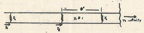
Let the radiators have an admittance  $Y_L$ , and let their spacing be  $\theta$  electrical degrees in the transmission line. Since the line is infinitely long, conditions at every radiator must be identical, so that  $Y_B = Y_A$ . Remembering this fact, and also that  $Y_O = 1$ , we may write
