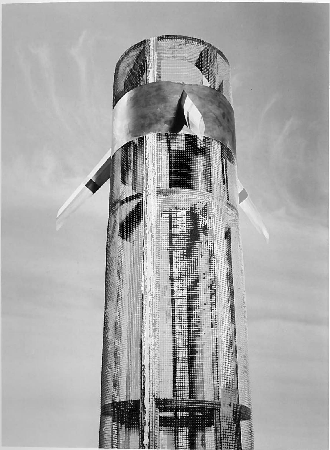
FIG. 13. FULL-SCALE MOCK-UP OF NOSE SECTION
