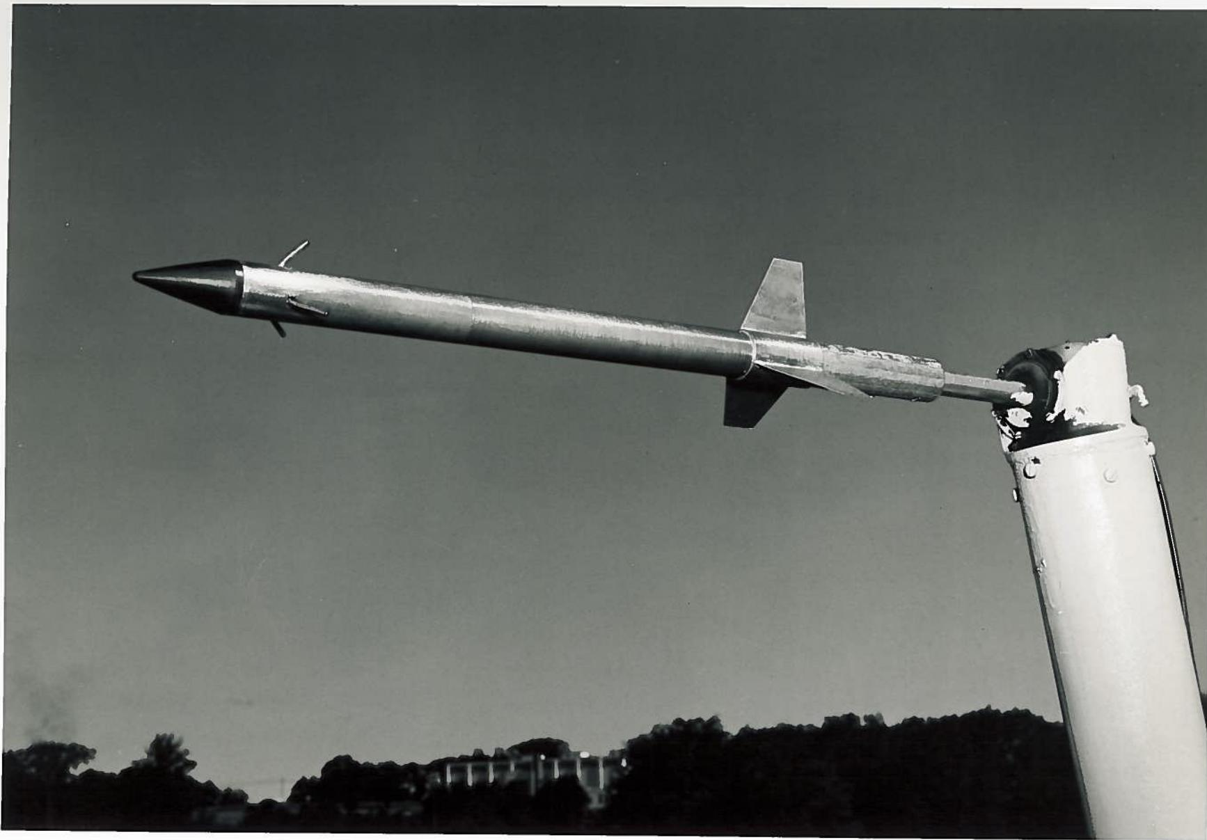
FIG. 1. SCALE MODEL MOUNTED FOR PATTERN MEASUREMENTS
