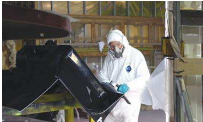
After the composite parts are cut they must be polished.
