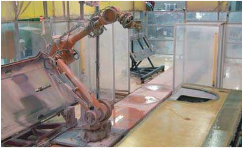
Robots use high-pressure water jets to cut and trim composite parts.
