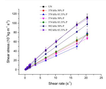
Fig. 2 Rheogram of unsonicated (UN) and sonicated (378, 574, and 992 kHz) bitumen at power input of 50 and 83.33 %
