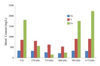
**Fig. 3** Metal content (ICP-MS analysis) of asphaltene extracted from bitumen sonicated under different frequencies and 50 % power input (UN: before sonication)
