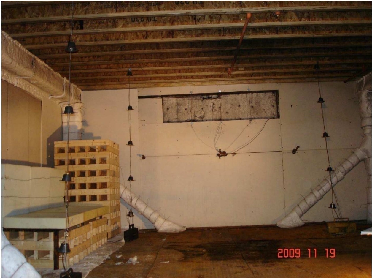
Figure 18. Sprinkler and CPVC piping relative to exposed wood I-joists and fuel package in Test PF-03C.
