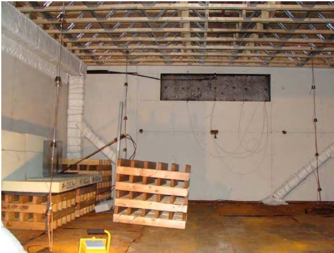
Figure 5. Layout of the fuel package in Test PF-06B.
