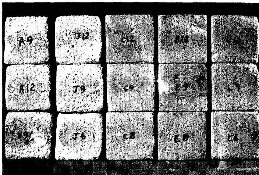
Figure 2 Bottom Surfaces - Same Mortars as in Figure 1 Note: Rounded edges and corners for A, H, and J cubes. Minor rounding of edges and broken corners for L cubes.
