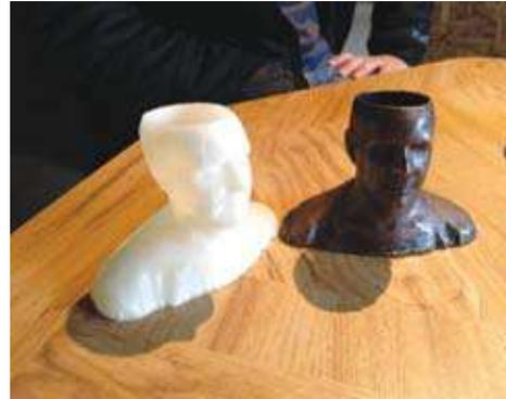
The rapid prototyper (3D printer) can quickly create prototypes to countless specifications.
