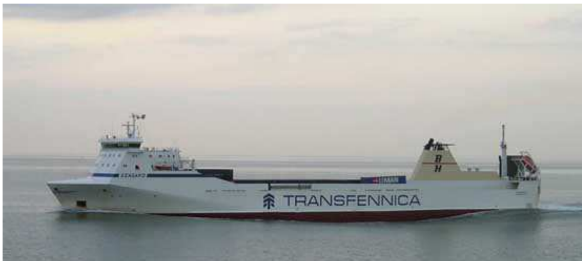
Figure C.2: Transfennica showing bow wave, water-surface drawdown and stern wave produced at 20 kt with 10 m under-keel clearance.
